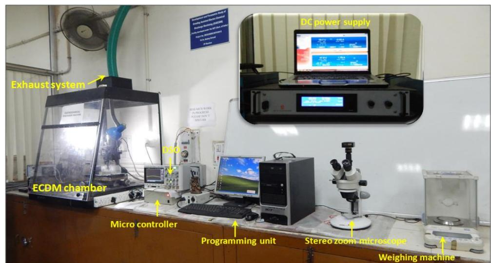
Figure 1. Pictorial view of ECSM machine.
