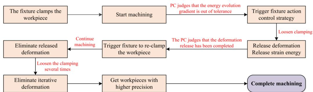
Figure 2. Control flow of floating clamping machining.
