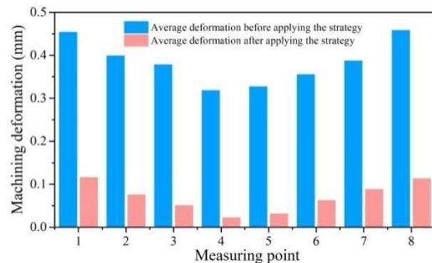
**Figure 13.** Comparison of the deformation before and after applying clamping control strategy.
