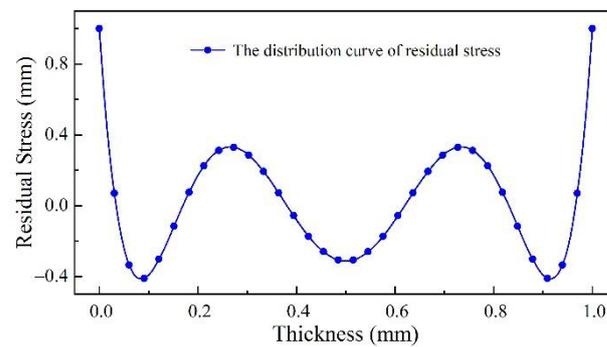
**Figure 4.** Initial residual stress model.
