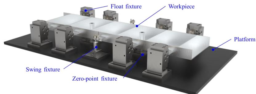
**Figure 9.** Floating clamping system.
