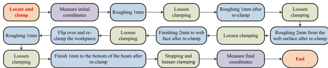
**Figure 10.** The process route of workpiece machining.
