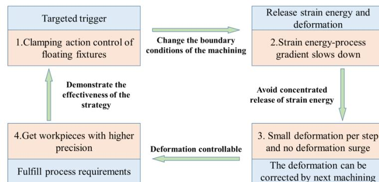
**Figure 1.** Principle of clamping action control based on gradient control of strain energy.
