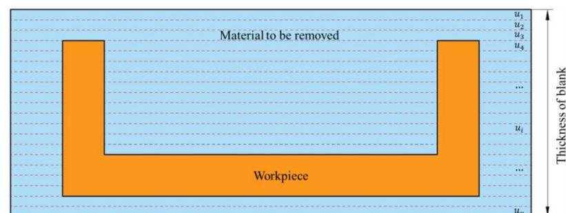
**Figure 3.** Schematic of material layer-by-layer milling.
