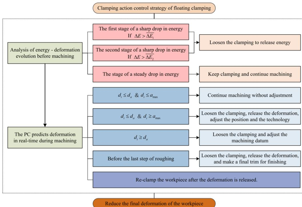
**Figure 6.** Clamping action control strategy for floating clamping machining.
