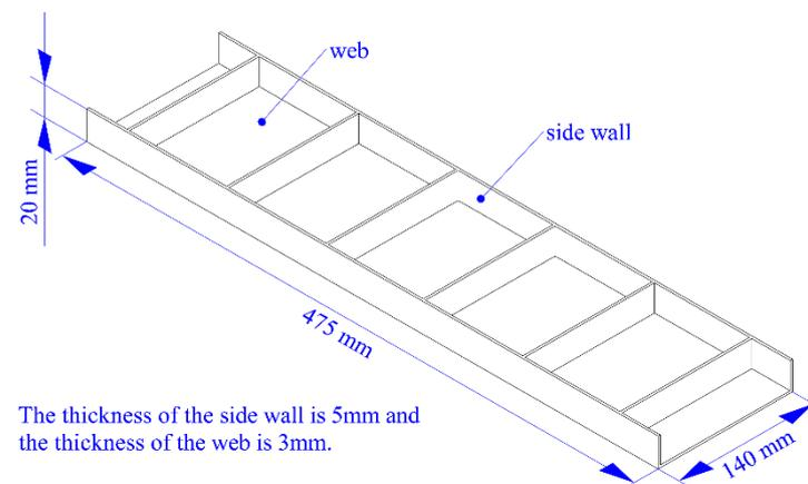
**Figure 8.** The structure and size of the thin-walled beam.
