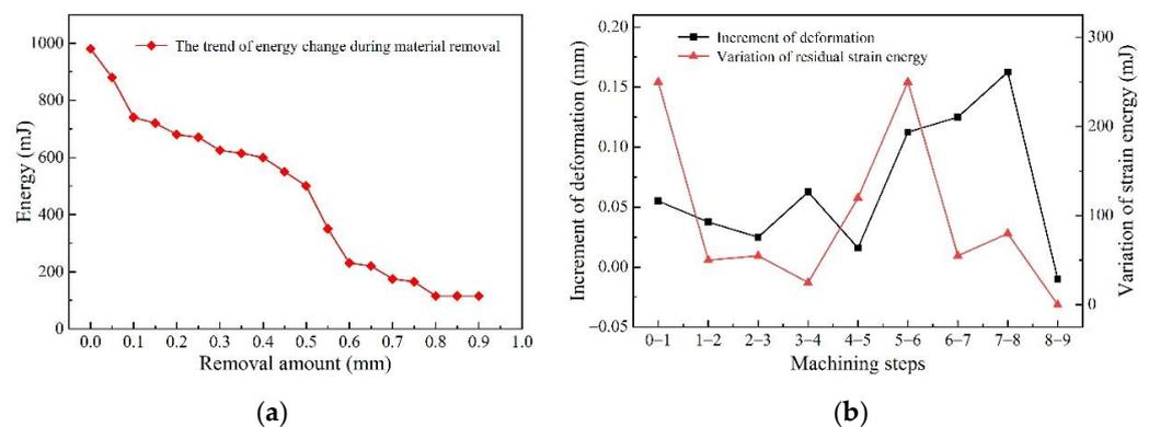
**Figure 5.** Variation of deformation and strain energy during machining: (a) relationship between strain energy and removal amount; (b) relationship between the increment of deformation and the variation of residual strain energy.
