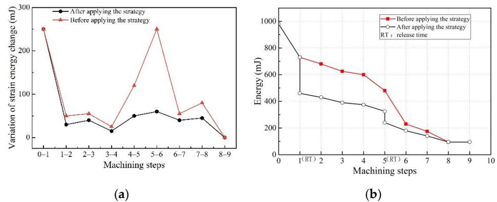
**Figure 7.** Effect of clamping control strategy on strain energy: (a) comparison of the variation of strain energy before and after applying clamping control strategy; (b) comparison of strain energy evolution process before and after applying clamping control strategy.
