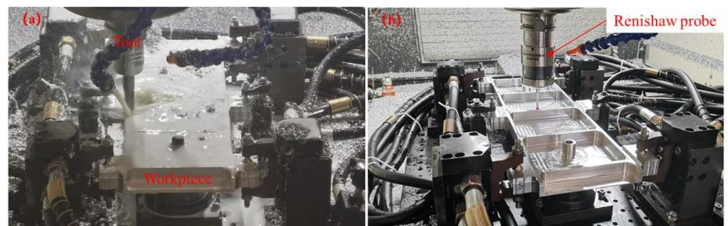
**Figure 11.** Experiment and measurement: (a) milling operation; (b) measuring deformation.
