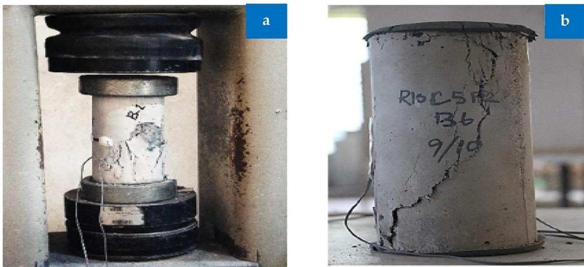
Figure 14. Cylinder failure under compression: (a) reference and (b) combination of RCA, rubber, and fibers [44]: used as per Elsevier permissions.
