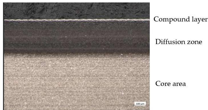
**Figure 8.** C 75 Stahl, nitrocarburized, etched with 3% Nital showing a dark etched diffusion zone with a compound layer and dark oxide layer.
