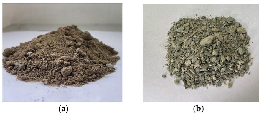
**Figure 1.** Appearance of sand used in this study: (a) SSTS; (b) M-S.
