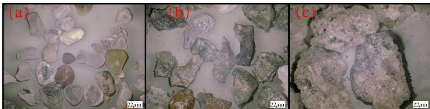
**Figure 4.** Ultra-deep field body microscopy images of materials: (a) washed SSTS with particle size of 0.3–0.6 mm, (b) washed M-S with particle size in 0.3–0.6 mm, and (c) unwashed SSTS with particle over 1.18 mm.
