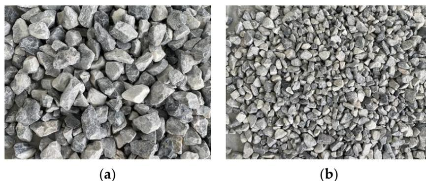
**Figure 5.** Appearance of the used coarse aggregate: (a) particle size in 10–25 mm; (b) particle size in 5–10 mm.
