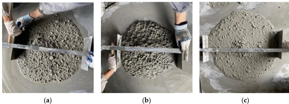
**Figure 9.** Appearance of concrete mixture of C30 strength grade. (a) C30DMS. (b) C30WMS. (c) C30M-S.
