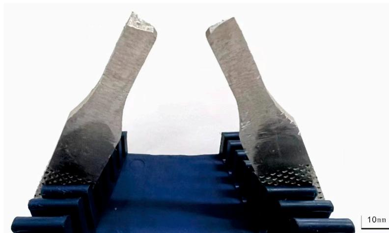
**Figure 5.** Fatigue fracture morphology of specimen No. 1 of dissimilar lightweight materials welded joints.
