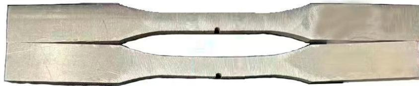
**Figure 2.** Comparison of deformed specimens of dissimilar lightweight materials welded joints with and without impact.
