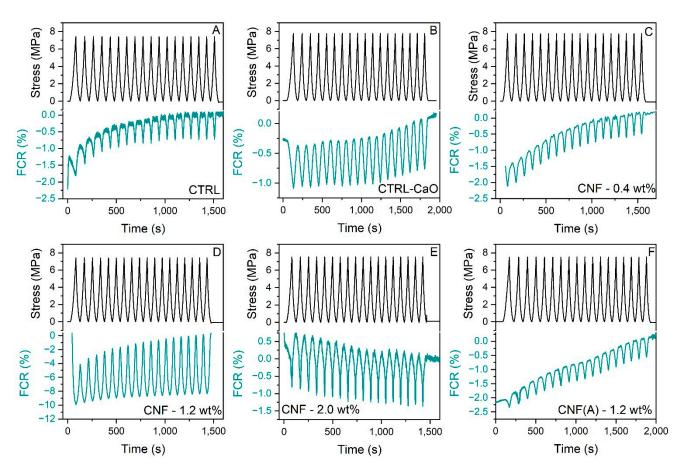
**Figure 9.** Piezoresistive behaviours of mortars under cyclic compressive loading. (**A**) Control mortar; (**B**) control mortar with CaO substrate; (**C**) mortar with 0.4 wt% of CNF; (**D**) mortar with 1.2 wt% CNF; (**E**) mortar with 2.0 wt%; (**F**) mortar with 1.2 wt% washed CNF.
