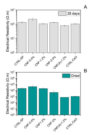
**Figure 7.** Effect of CNF concentration on the electrical resistivity of mortar specimens (**A**) immediately after 28 days in a high-humidity chamber and (**B**) after drying.
