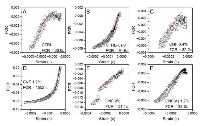
**Figure 10.** FCR versus strain for mortar specimens at different CNF concentrations under a monotonic uniaxial compressive loading with an amplitude of 7.5 MPa. (A) Control mortar; (B) control mortar with CaO substrate; (C) mortar with 0.4 wt% of CNF; (D) mortar with 1.2 wt% CNF; (E) mortar with 2.0 wt%; (F) mortar with 1.2 wt% washed CNF.
