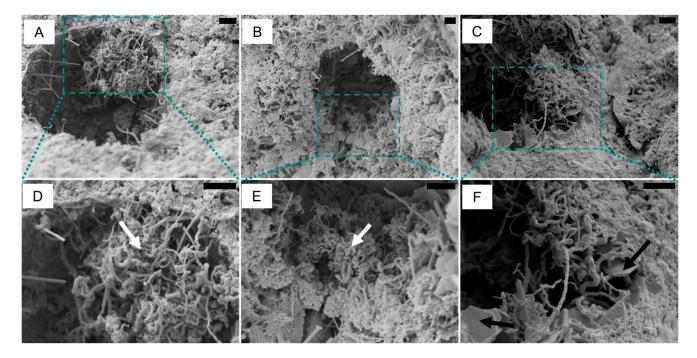
**Figure 6.** Scanning electron microscopy of carbon nanofibers supported in CaO, dispersed in mortar. Scale bar 2  $\mu$ m. (A–C) mortar surface containing the nest of CNF; (D–F) details of the CNF next, white arrows indicate CNF and black arrow indicate portlandite.
