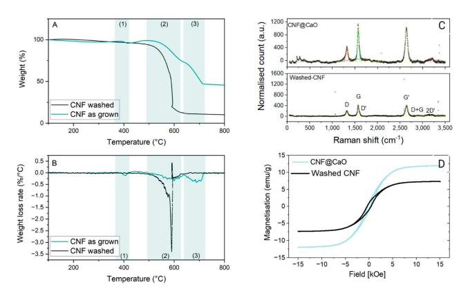
**Figure 5.** Characterisation of CNF@CaO as produced and CNF after acid washing. (**A**) Thermogravimetric analysis of as-grown CNF in the surface of CaO (teal) and acid-washed nanomaterial, purified for the removal of CaO (black); (**B**) Weight loss rate for the as-grown CNF (purple) and purified CNF (teal); (**C**) Raman spectra of CNF@CaO (top) and CNF—washed (bottom); (**D**) Magnetisation curve of CNF@CaO (teal) and CNF—washed (black).
