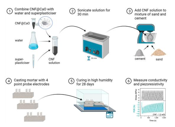
**Figure 2.** Workflow used for dispersion of CNF in mortar, followed by measurement of electrical properties.
