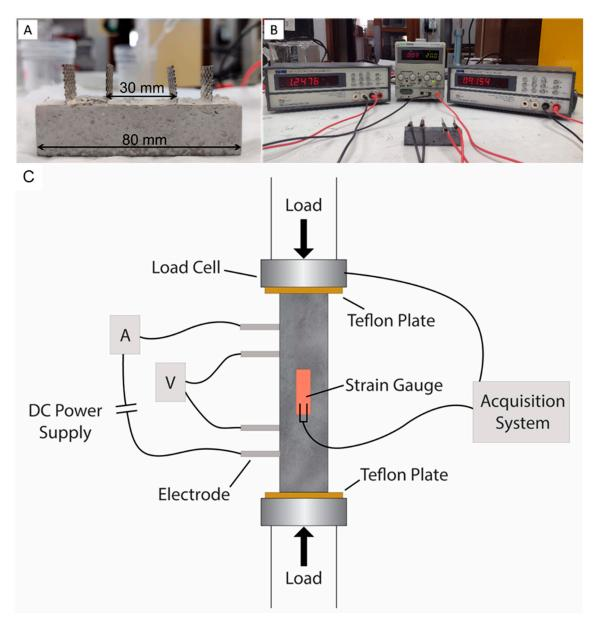
**Figure 3.** Set-up for measuring the conductivity of the samples. (**A**) Mortar sample with 4 electrodes; (**B**) multimeters for measurements; (**C**) experimental set-up used to measure the piezoresistive behaviour of the mortar samples containing CNF.
