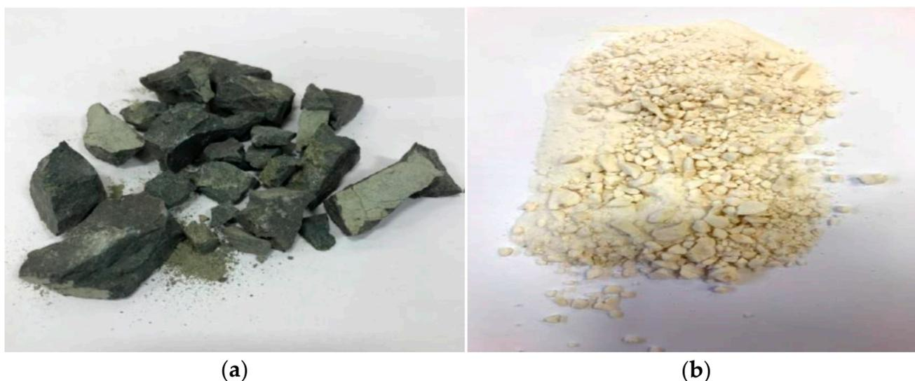
**Figure 1.** Natural raw materials from the Lower Silesia region of Poland used to melt glasses, (a) amphibolite, (b) dolomite.
