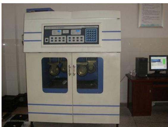
**Figure 5.** Wheel-tracking test device.
