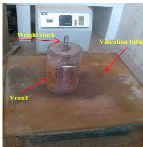
**Figure 4.** Vibrating compaction test device.
