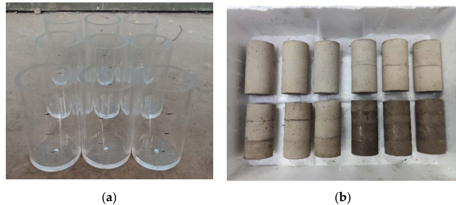
Figure 2. Filling Mold and Filling Body Sample; (a) Filling Mold, (b) Filling Body Sample.
