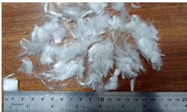
Figure 1. Polypropylene fibers supplied by Viapol.
