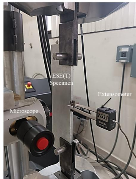
**Figure 2.** Experimental test setup for the crack propagation.
