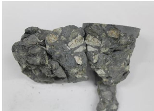
**Figure 1.** Fracture surface showing cracking through aggregate particles in geopolymer concrete.
