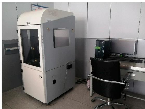
Figure 3. MFT-5000 friction and wear test bench.
