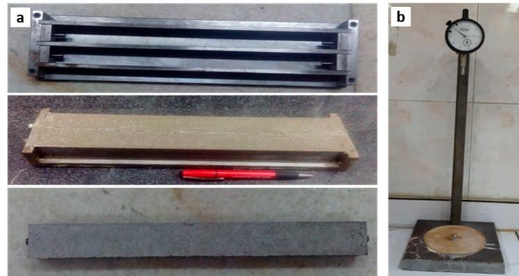
**Figure 1.** Accelerated mortar bar samples (ASTM C 1260): (a) casting equipment and mortar bars; (b) length measurement facility.
