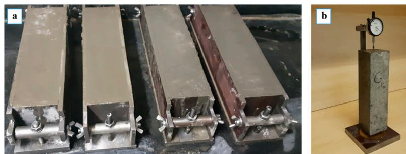
**Figure 2.** Concrete prism samples: (a) casting; (b) length measuring facility.
