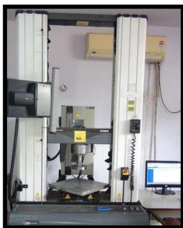
Figure 5. INSTRON 3382 series operating on Bluehill software Universal Testing Machine.
