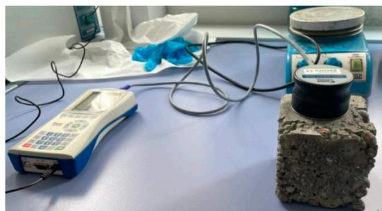
**Figure 4.** Experimental setup of the thermal conductivity test.
