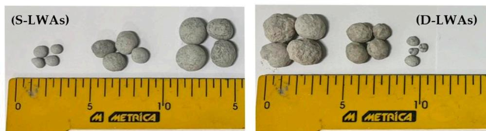
**Figure 1.** Single lightweight artificial aggregates (S-LWAs) and double lightweight artificial aggregates (D-LWAs).
