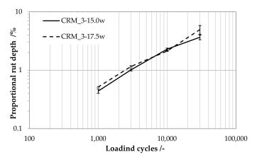
**Figure 9.** Proportional rut depth as a function of loading cycles at 20 °C.
