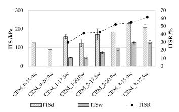
**Figure 8.** Indirect tensile strength (ITS<sub>d</sub> in dry conditions, ITS<sub>w</sub> after soaking) and strength ratio (ITSR) at 20  $^{\circ}$ C.
