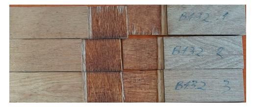
**Figure 12.** Scheme of the plywood specimen for the test (A) and experimentally obtained plywood specimen after the shear strength test.
