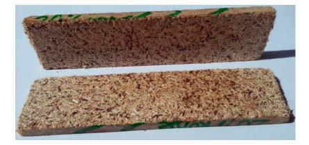
Figure 10. Particleboard specimens before bending test.
