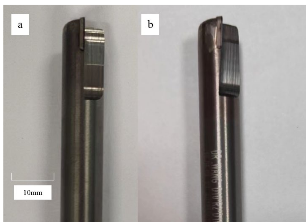
Figure 2. Cutting tools. (a) PCD tool with 0° rake angle; (b) PCD tool with 4° rake angle.
