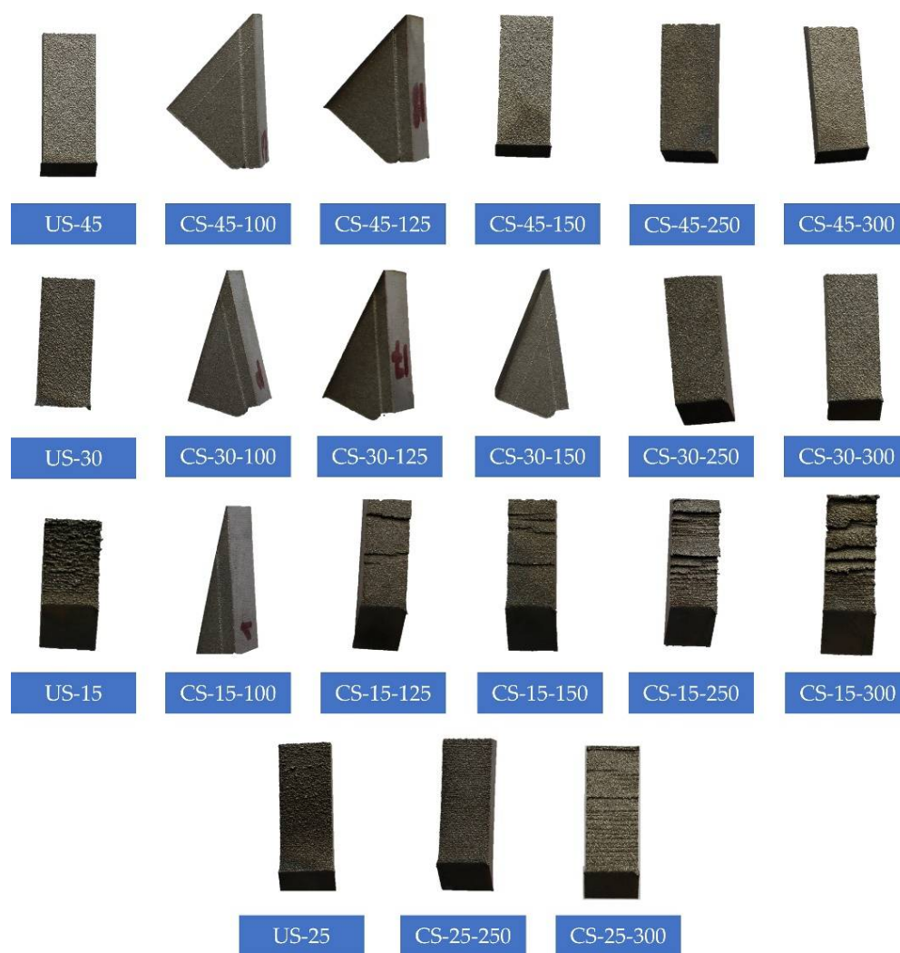
Figure 2. Contact-free supported geometries printed via DMLM (Coupons like pyramids are the ones that fused to support. Remaining ones represent overhang areas of corresponding coupons).
