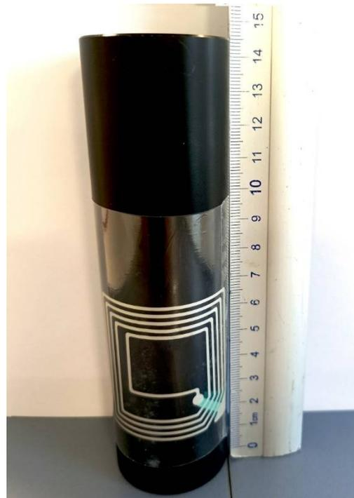
**Figure 7.** NFC antenna printed on shrink sleeve label applied on the container.
