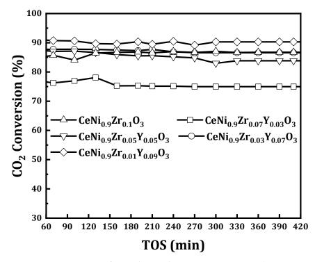
**Figure 7.** CO<sub>2</sub> conversion of perovskite catalysts CeNi<sub>0.9</sub>Zr<sub>0.1-x</sub>Y<sub>x</sub>O<sub>3</sub> (x = 0, 0.03, 0.05, 0.07, and 0.09) at 800 °C, 1 atmosphere and GHSV = 42 L/(h.g<sub>cat</sub>).
