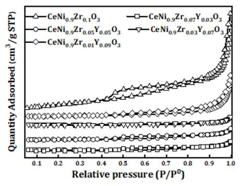
**Figure 1.** Nitrogen physisorption isotherms of perovskite catalyst CeNi<sub>0.9</sub> $Zr_{0.1-x}Y_xO_3$  (x = 0, 0.03, 0.05, 0.07, and 0.09).
