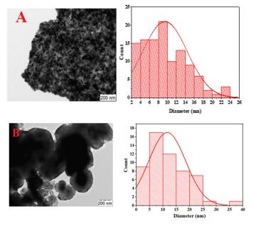
**Figure 5.** TEM micrographs and matching particle size distribution for fresh  $CeNi_{0.9}Zr_{0.1}O_{3.}$  (**A**) and used  $CeNi_{0.9}Zr_{0.1}O_{3.}$  (**B**) catalyst.
