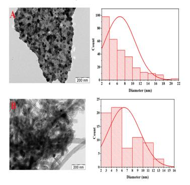
**Figure 6.** TEM micrographs and matching particle size distribution for fresh  $CeNi_{0.9}Zr_{0.01}Y_{0.09}O_3$ . (A) and used  $CeNi_{0.9}Zr_{0.01}Y_{0.09}O_3$ . (B) catalyst.
