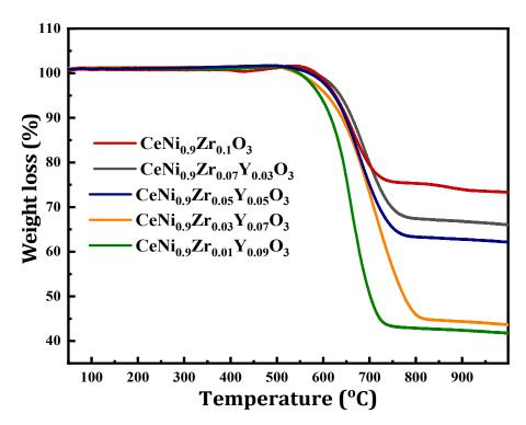
**Figure 10.** TGA Curves of perovskite catalysts  $\text{CeNi}_{0.9}\text{Zr}_{0.1-x}\text{Y}_x\text{O}_3$  (x = 0, 0.03, 0.05, 0.07, and 0.09) at 800 °C.
