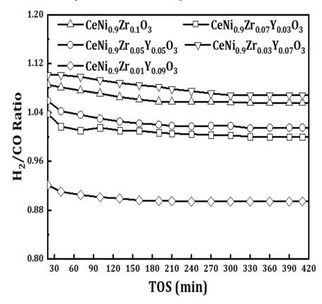
**Figure 9.**  $H_2/CO$  ratio of perovskite catalysts CeNi<sub>0.9</sub>Zr<sub>0.1-x</sub>Y<sub>x</sub>O<sub>3</sub> (x = 0, 0.03, 0.05, 0.07, and 0.09) at 800 °C, 1 atmosphere and GHSV = 42 L/(h.g<sub>cat</sub>).
