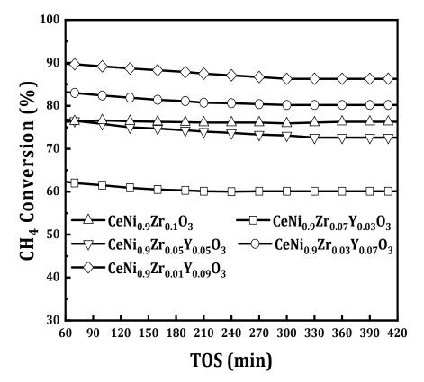
**Figure 8.** CH<sub>4</sub> conversion of perovskite catalysts CeNi<sub>0.9</sub>Zr<sub>0.1-x</sub>Y<sub>x</sub>O<sub>3</sub> (x = 0, 0.03, 0.05, 0.07, and 0.09) at 800 °C, 1 atmosphere and GHSV = 42 L/(h.g<sub>cat</sub>).
