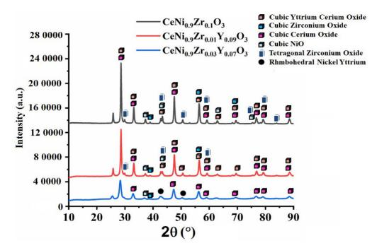
**Figure 3.** XRD pattern of perovskite catalyst CeNi<sub>0.9</sub>Zr<sub>0.1-x</sub> $Y_xO_3$  (x = 0.00, 0.07 and 0.09).
