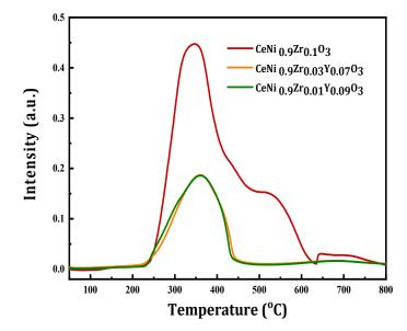
**Figure 2.** H<sub>2</sub>-TPR profiles of perovskite catalyst CeNi<sub>0.9</sub>Zr<sub>0.1-x</sub> $Y_xO_3$  (x = 0, 0.07 and 0.09).
