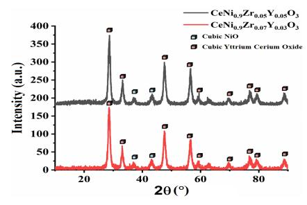
**Figure 4.** XRD pattern of perovskite catalyst CeNi<sub>0.9</sub>Zr<sub>0.1-x</sub>Y<sub>x</sub>O<sub>3</sub> (x = 0.03 and 0.05). **Table 2.** Summary of Nickel Particle Size Derived from TEM Analysis.
