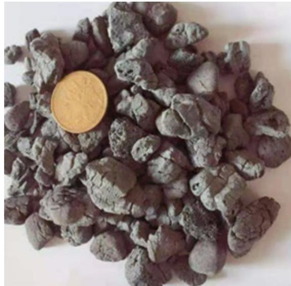
**Figure 1.** Artificial lightweight shale ceramsite with size of 5–15 mm.
