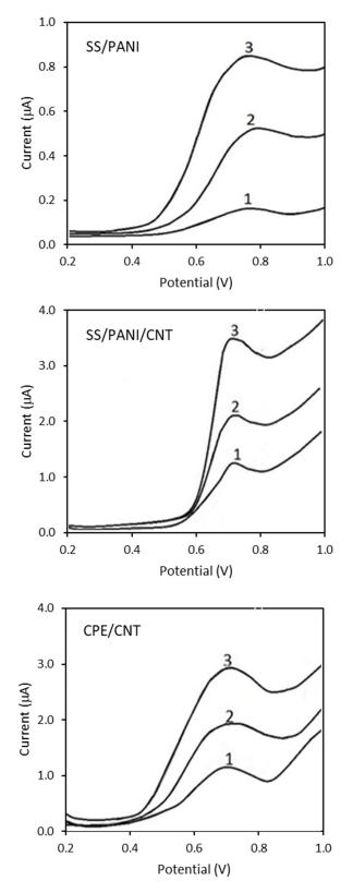
**Figure 8.** Differential pulse voltammograms registered for 0.5 mmol/L 4-CP in 0.1 mol/L solutions of Na<sub>2</sub>SO<sub>4</sub> on SS/PANI and SS/PANI/CNT electrodes obtained after 1–10 cycles, 2–20 cycles, 3–30 cycles, as well as on CPEs modified with CNTs content of 1–2.5%, 2–5%, and 3–10%.
