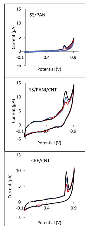
**Figure 7.** Cyclic voltammograms registered for 0.5 mmol/L 4-CP in 0.1 mol/L solutions of Na<sub>2</sub>SO<sub>4</sub> on SS/PANI and SS/PANI/CNT electrodes obtained after 10 cycles ---, 20 cycles ---, 30 cycles ---, as well as on CPEs modified with CNTs content of 2.5% ---, 5% ---, and 10% ---.
