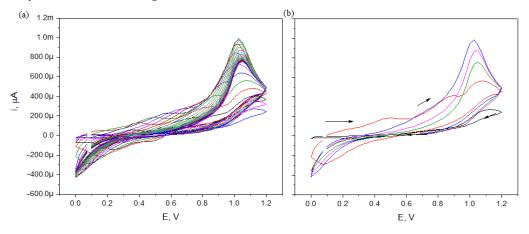
**Figure 3.** The CV curves registered for 0.2 mol/L aniline in 0.5 mol/L  $H_2SO_4$  solutions using stainless steel wire electrodes after 1–30 cycles (**a**) and chosen for ---- 1, ---- 5, ---- 10, ---- 20, ---- 30 cycles (**b**).
