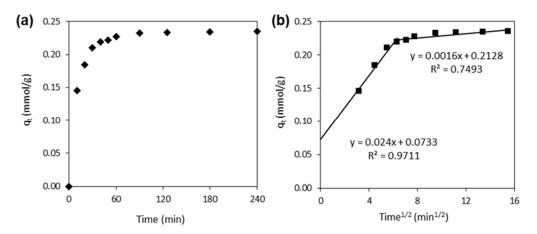
**Figure 2.** (**a**) The adsorption kinetics of 4-CP onto CNTs, and (**b**) the intraparticle diffusion kinetic model.
