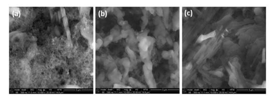
**Figure 5.** The SEM images of the stainless steel fiber coated with PANI/CNT layers after 10 (**a**), 20 (**b**), and 30 (**c**) CV cycles.
