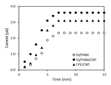
**Figure 6.** The effect of accumulation time on the peak current of the 0.5 mmol/L 4-CP in 0.1 mol/L  $Na_2SO_4$  solutions.
