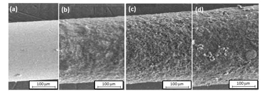
**Figure 4.** The SEM image of the stainless steel fiber before the electropolymerization (**a**) and after 10 (**b**), 20 (**c**), and 30 (**d**) cycles.
