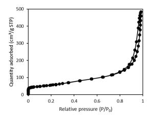
Figure 1. Nitrogen adsorption-desorption isotherm of CNTs at 77.4 K.
