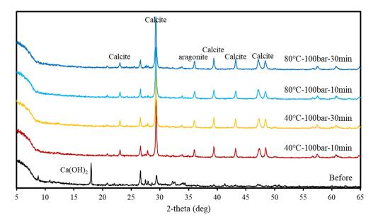
Figure 7. XRD patterns obtained at 100 bar.
