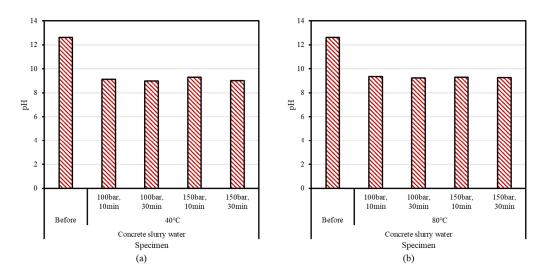
**Figure 5.** Results of pH measurements for supercritical CO<sub>2</sub> carbonation at (a) 40  $^{\circ}$ C or (b) 80  $^{\circ}$ C.
