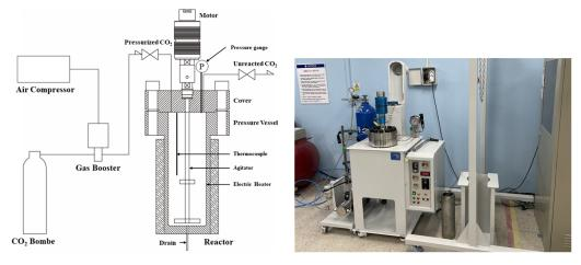
Figure 3. Schematic and photograph of the supercritical CO<sub>2</sub> reactor.
