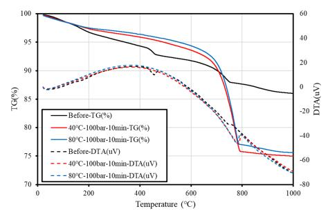
Figure 9. TG-DTA results obtained before and after supercritical CO<sub>2</sub> carbonation.
