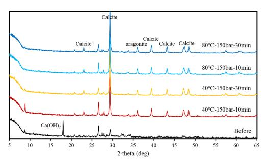
Figure 8. XRD patterns obtained at 150 bar.
