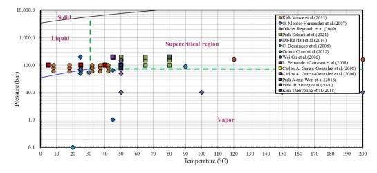
**Figure 1.** Temperature–pressure conditions reported in the current literature on supercritical CO<sub>2</sub> mineral carbonation.
