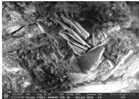
Figure 21. Microstructure of ZV mortar (FBC II) after 90 days of curing in seawater solution.
