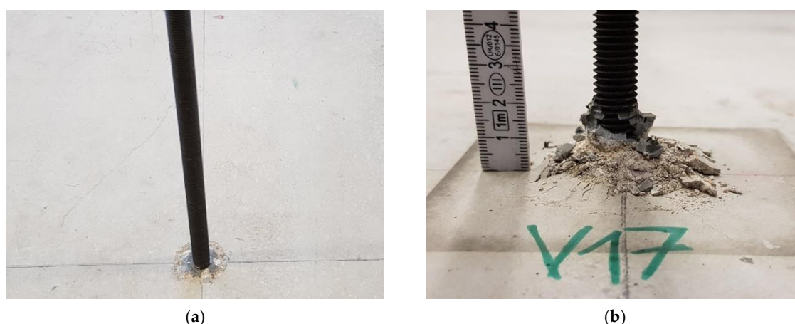
Figure 4. Overview of the bonded anchor system used in the test series. (a) installation of anchor system; (b) typical failure mode.
