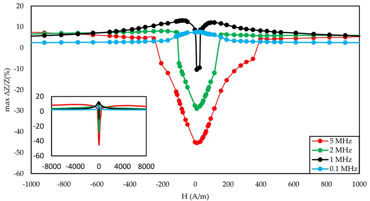
**Figure 5.** Dependence of max change of impedance ratio in a function of magnetizing field for different driving frequencies for the as-cast sample.
