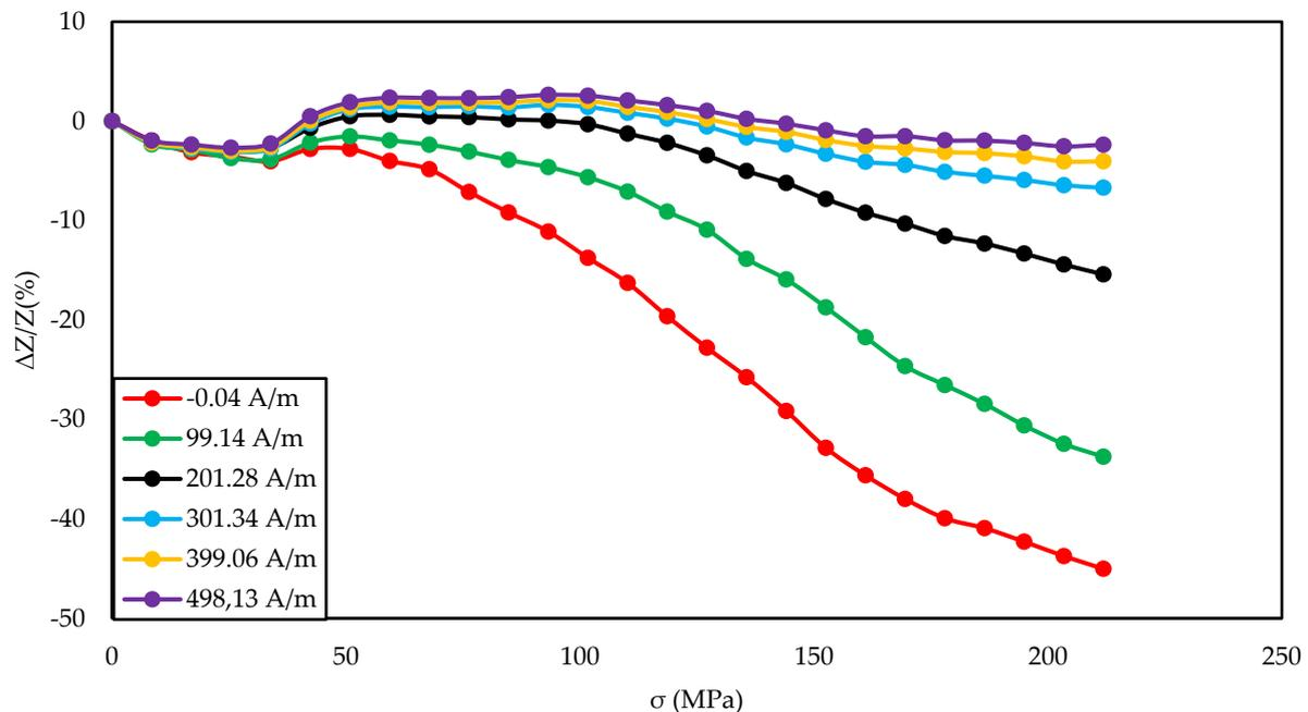
**Figure 3.** Dependence of impedance in a function of stresses for different magnetizing fields for the as-cast sample.
