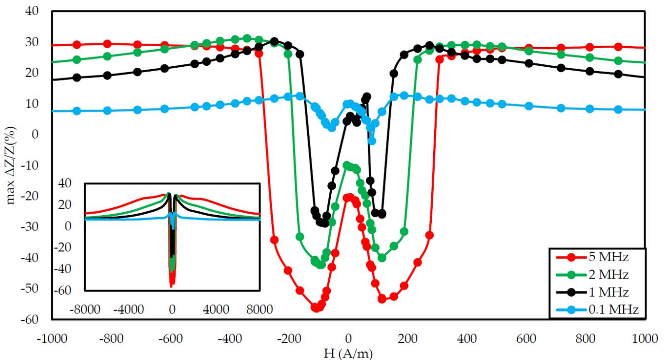
**Figure 11.** Dependence of max change of impedance ratio in a function of magnetizing field for different driving frequencies for the annealed by a 900 mA current sample.
