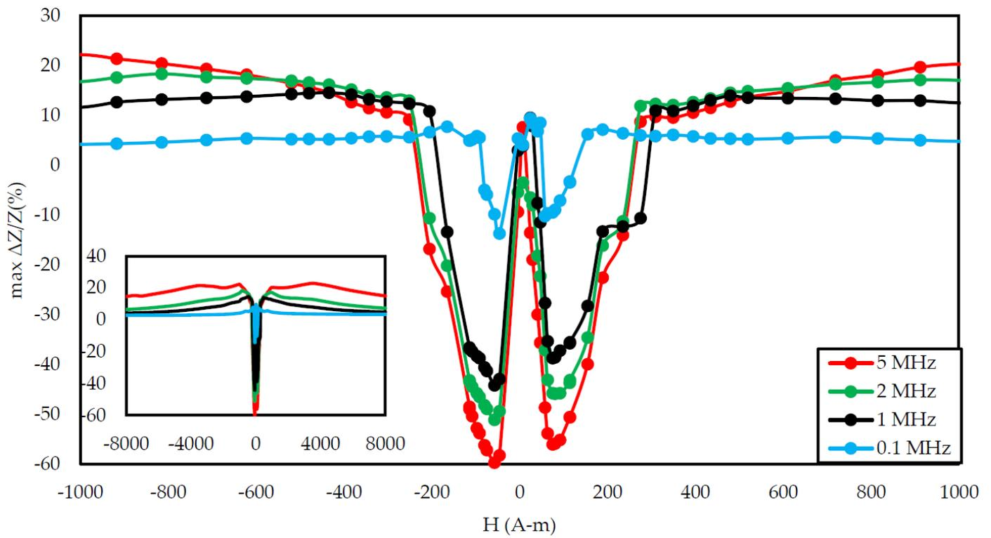
**Figure 8.** Dependence of max change of impedance ratio in a function of magnetizing field for different driving frequencies for the annealed by a 700 mA current sample.
