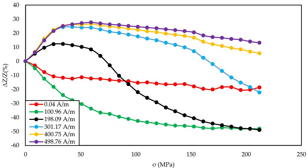
**Figure 9.** Dependence of impedance in a function of stresses for different magnetizing fields for the annealed by a 900 mA current sample.
