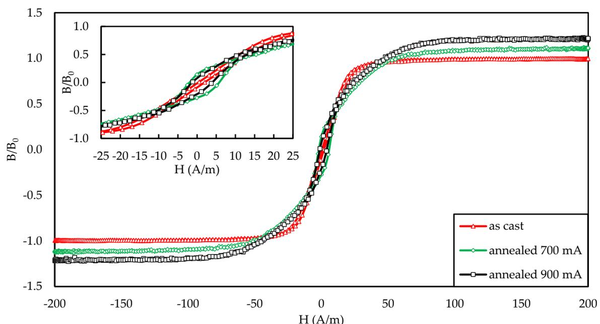
**Figure 1.** Hysteresis loop of as-cast and annealed samples used in the study.
