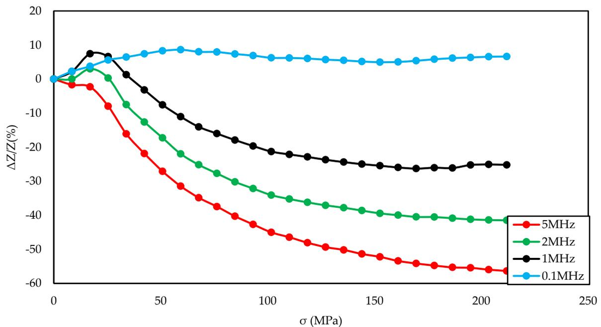
**Figure 10.** Dependence of impedance in a function of stresses for different driving frequencies for the annealed by a 900 mA current sample and  $-110$  A/m magnetizing field.
