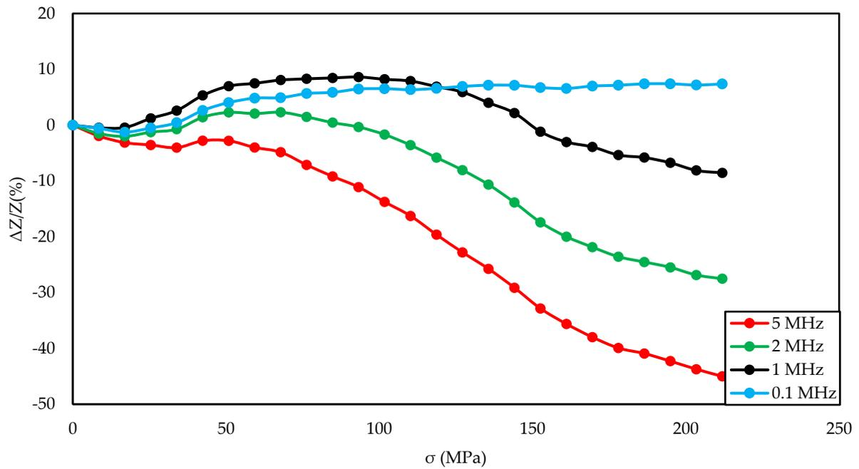
**Figure 4.** Dependence of impedance in a function of stresses for different driving frequencies for the as-cast sample and 0 A/m magnetizing field.
