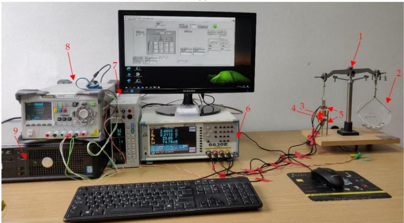
**Figure 2.** Developed test stand: (a) block diagram of the developed stand; (b) photo of the developed stand for testing stress-impedance in a function of the external magnetic field. The diagram and the photo contains: 1—balance scale, 2—applied mass, 3—magnetizing coil, 4—tested sample, 5—electrodes/measuring holders, 6—high-frequency RLC bridge, 7—ammeter, 8—laboratory power supply, 9—PC computer.
