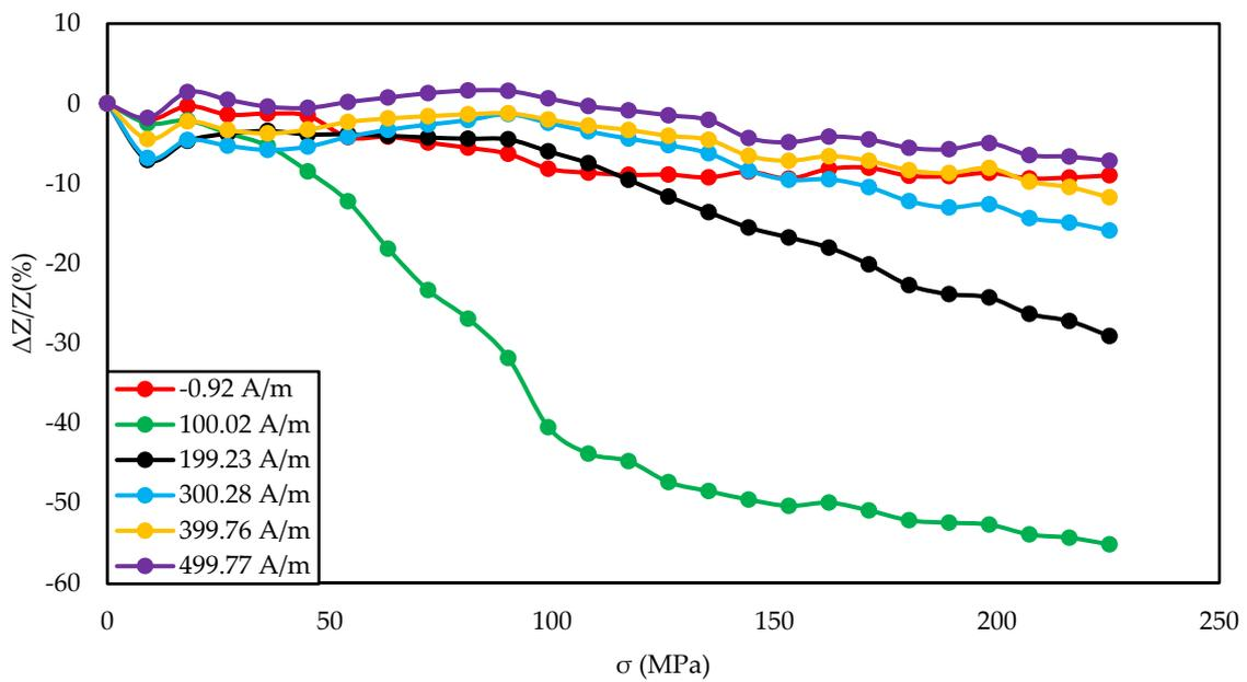
**Figure 6.** Dependence of impedance in a function of stresses for different magnetizing fields for the annealed by a 700 mA current sample.
