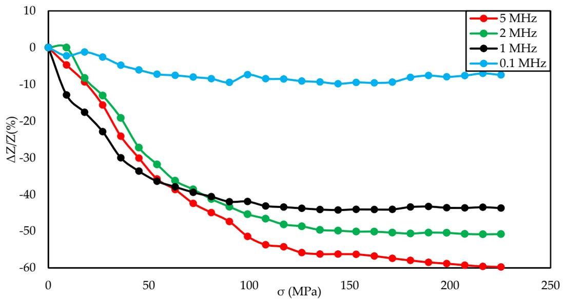
**Figure 7.** Dependence of impedance in a function of stresses for different driving frequencies for the annealed by a 700 mA current sample and  $-60$  A/m magnetizing field.
