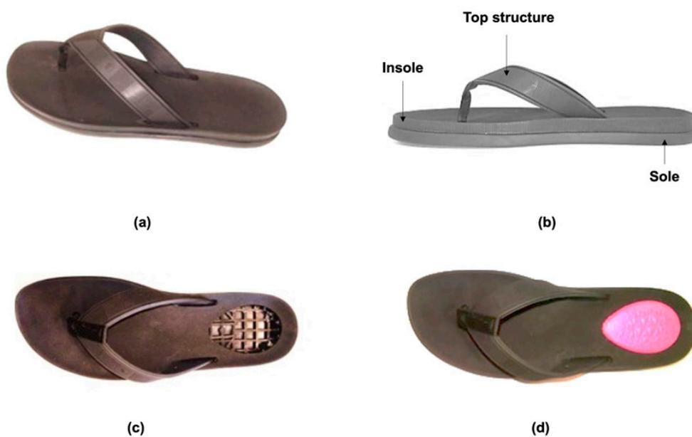
**Figure 11.** Slippers used in the case study: (a) original TPU slipper; (b) structure of the slippers; (c) prototype slipper with a cut in the insole heel zone for insert placement; (d) prototype slipper with insert.
