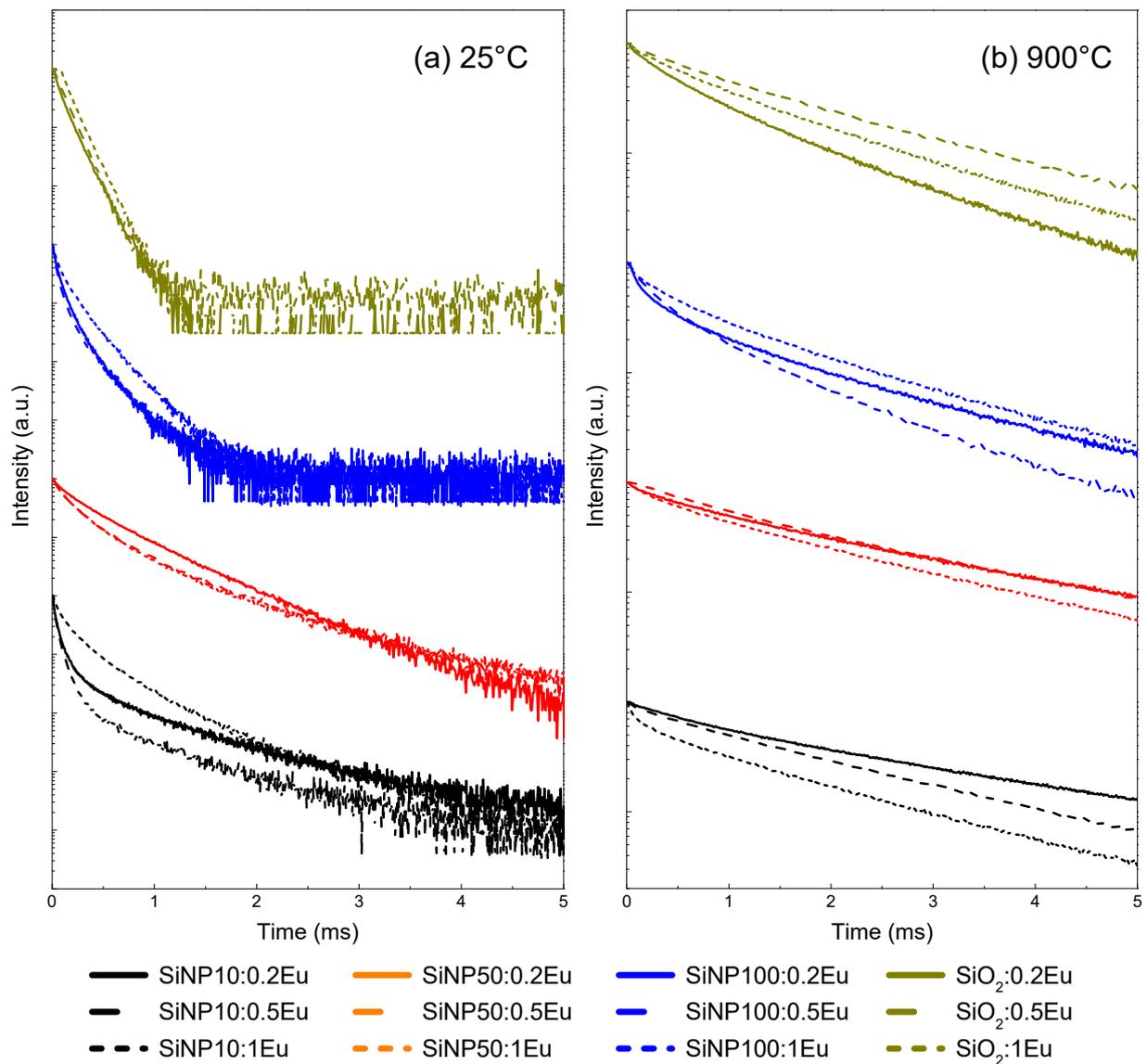
**Figure 6.** Luminescence decays of level  $^5D_0$  of  $\text{Eu}^{3+}$  measured at the maximum intensity of the emission band  $^5D_0 \rightarrow ^7F_2$  in Eu-doped silica nanoparticles and bulk: (a) before thermal treatment at  $900\text{ }^\circ\text{C}$ ; and (b) after thermal treatment at  $900\text{ }^\circ\text{C}$ .
