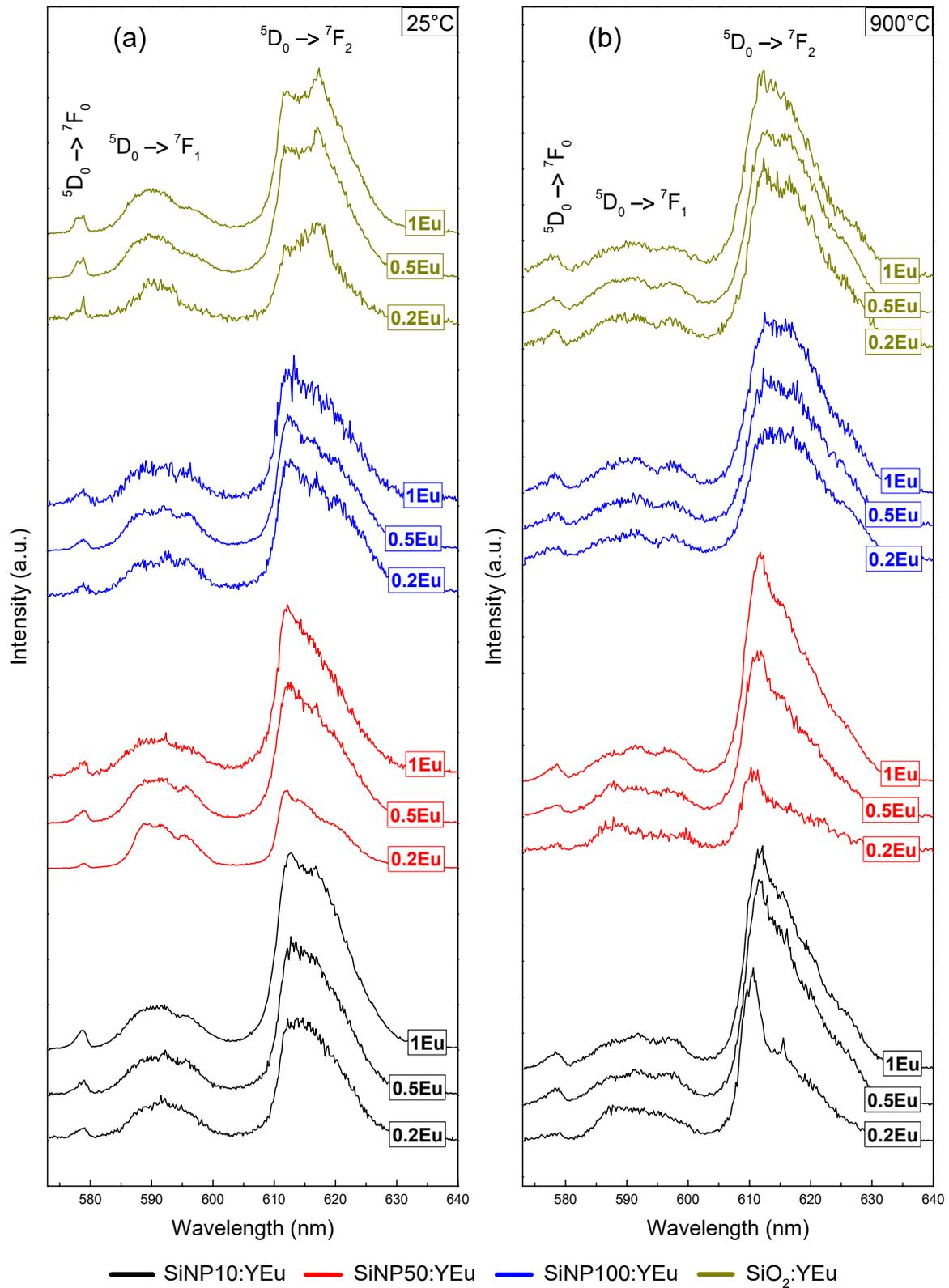
**Figure 5.** Emission spectra obtained under pulsed laser excitation at 532 nm at room temperature of Eu-doped silica nanoparticles and bulk (a) before and (b) after thermal treatment at 900 °C (the intensities are normalized to the maximum of the emission band  ${}^5\text{D}_0 \rightarrow {}^7\text{F}_1$ ).
