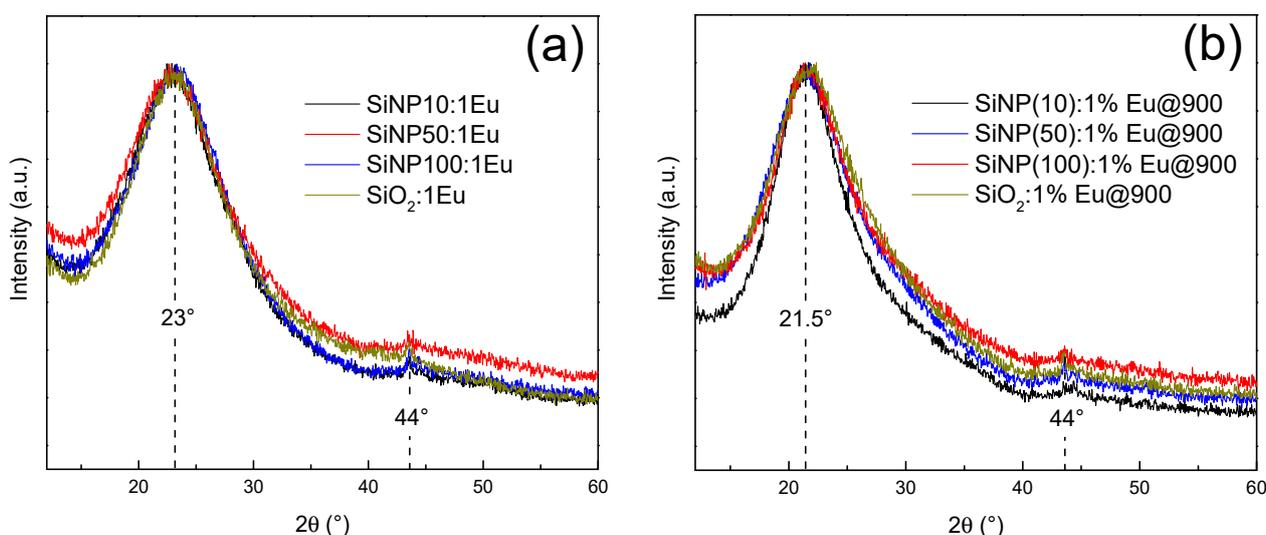
**Figure 3.** XRD patterns of SiNPX:1Eu and of bulk SiO<sub>2</sub>:1Eu: (a) before thermal treatment; and (b) after thermal treatment.
