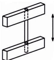
**Figure 1.** Illustration of the “H” type specimen. A silver wire fixed in two rubber plates during their crosslinking.
