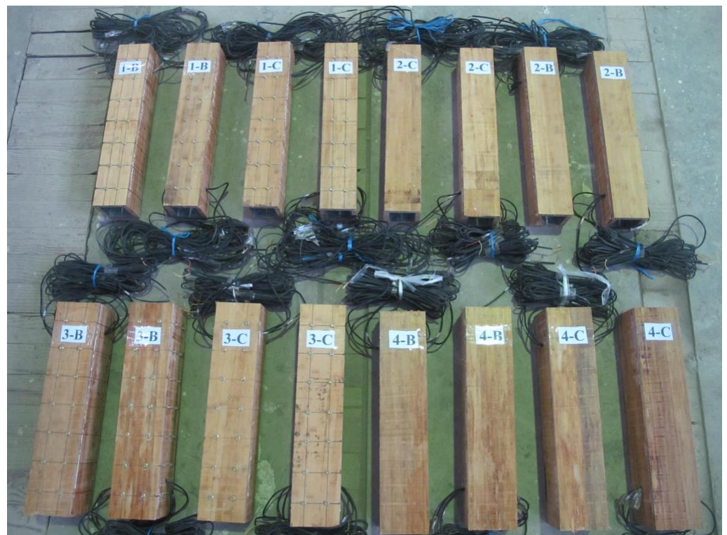
Figure 2. Specimens of composite column.
