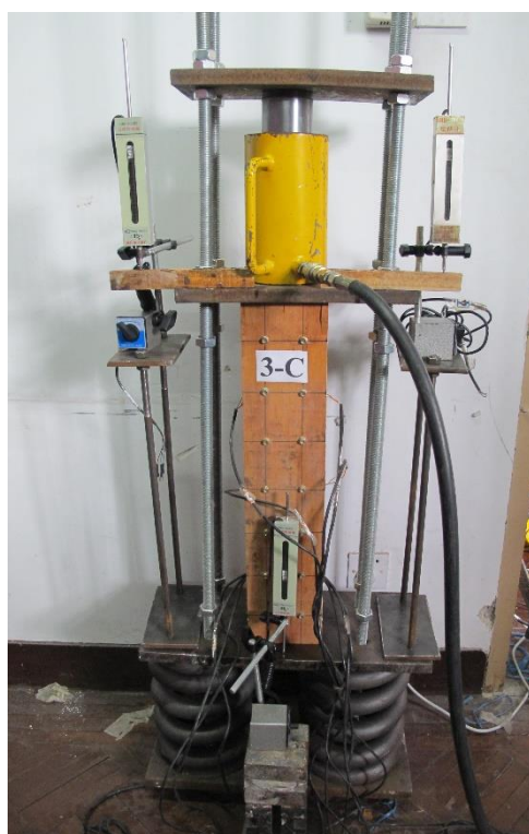
Figure 3. Device for long-term loading.
