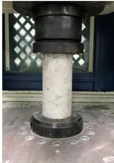
**Figure 3.** Compression test of carbon-fiber-reinforced concrete (CFRC) cylindrical specimen.
