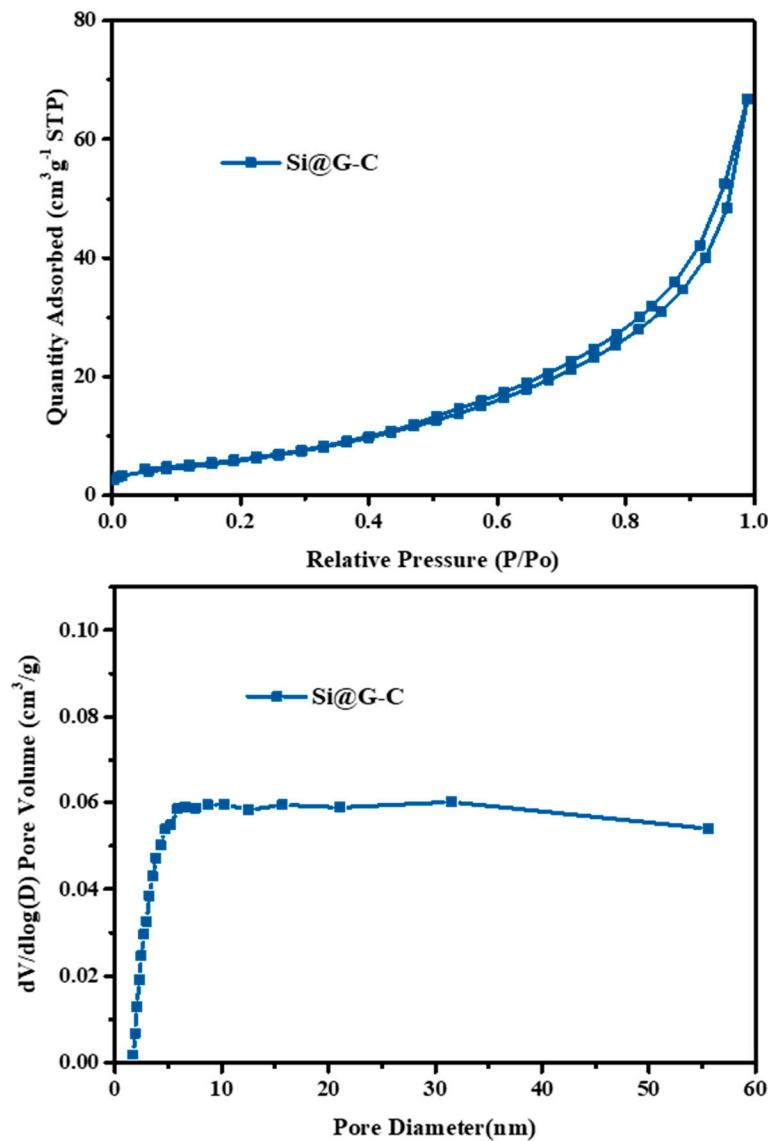
**Figure S6.** The BET results of the Si @G-C (a,) The  $\text{N}_2$  absorption and desorption curves of the composites and (b) the corresponding pore size distribution.
