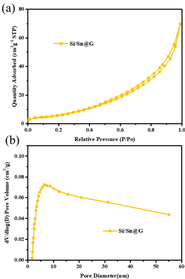
**Figure S5.** The BET results of the Si/Sn@G (a,) The  $\text{N}_2$  absorption and desorption curves of the composites and (b) the corresponding pore size distribution.
