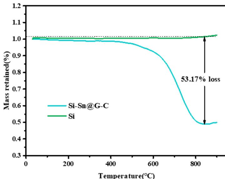
**Figure S2.** TGA curve of Si-Sn@G-C composite.
