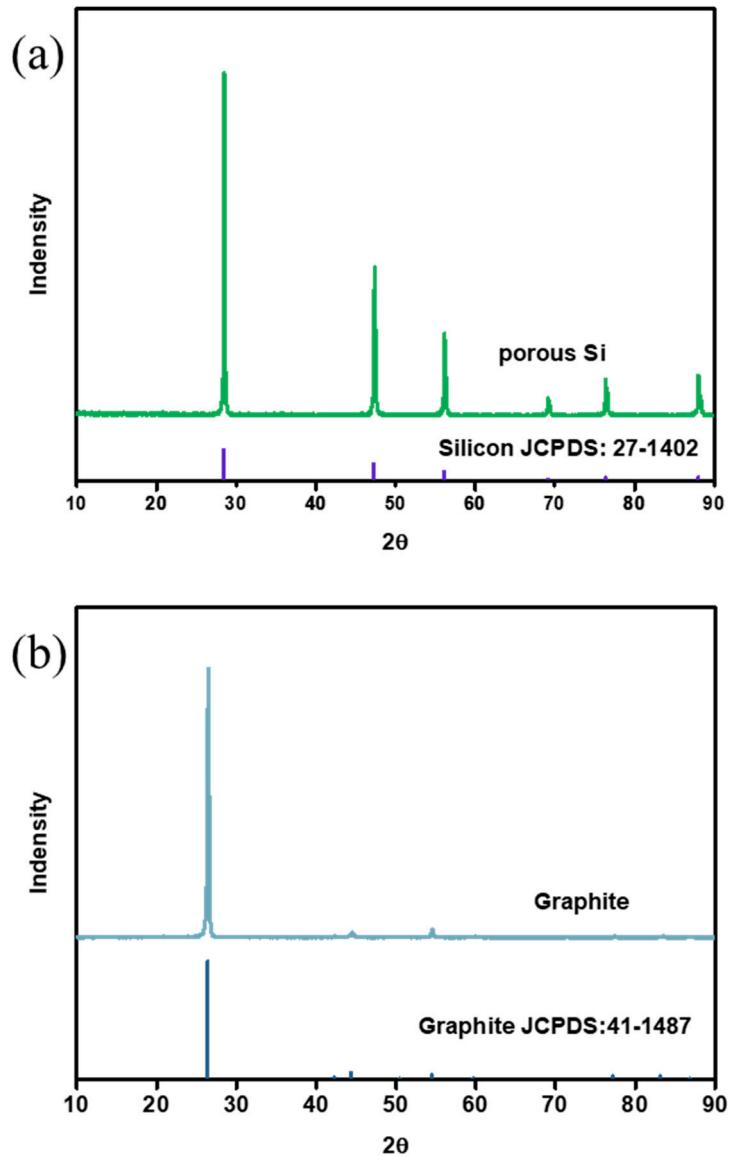
**Figure S1.** XRD pattern of (a) porous Si, (b) graphite.
