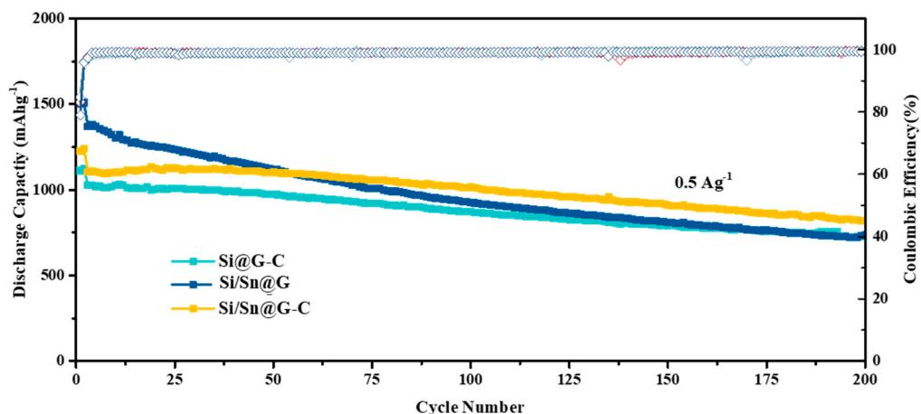
**Figure S8.** cycling performance at a current density of  $0.5 \text{ A g}^{-1}$  of Si/Sn@G-C, Si@G-C and Si/Sn@G anode.
