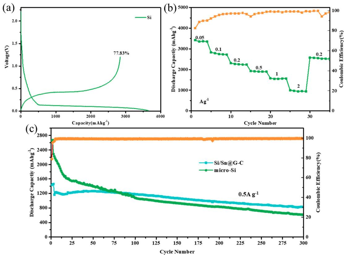
**Figure S7.** Electrochemical of micro sized porous Si (a) the charge/discharge profiles (b) the rate performance (c) the cycle performance
