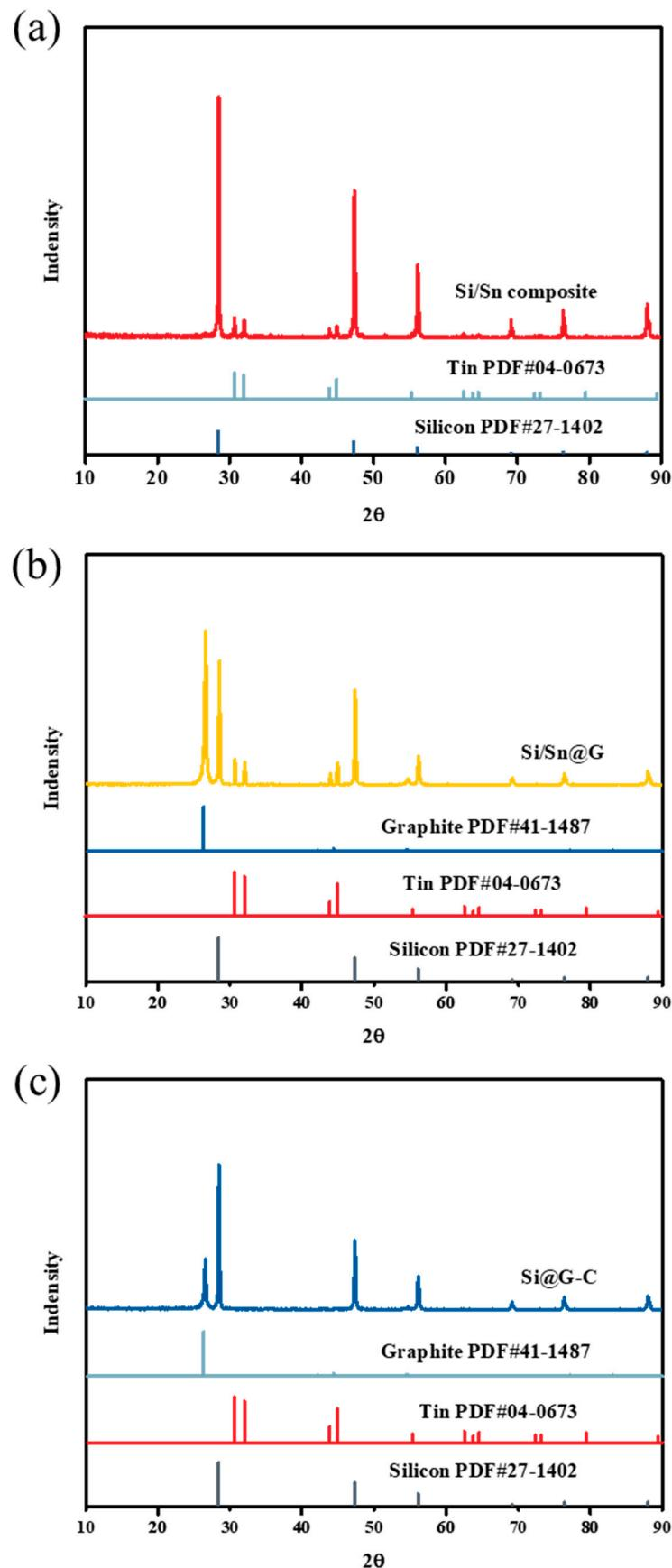
**Figure S3.** XRD pattern of (a) Si-Sn composite (b) Si/Sn@G composite and (c) Si@G-C composite.
