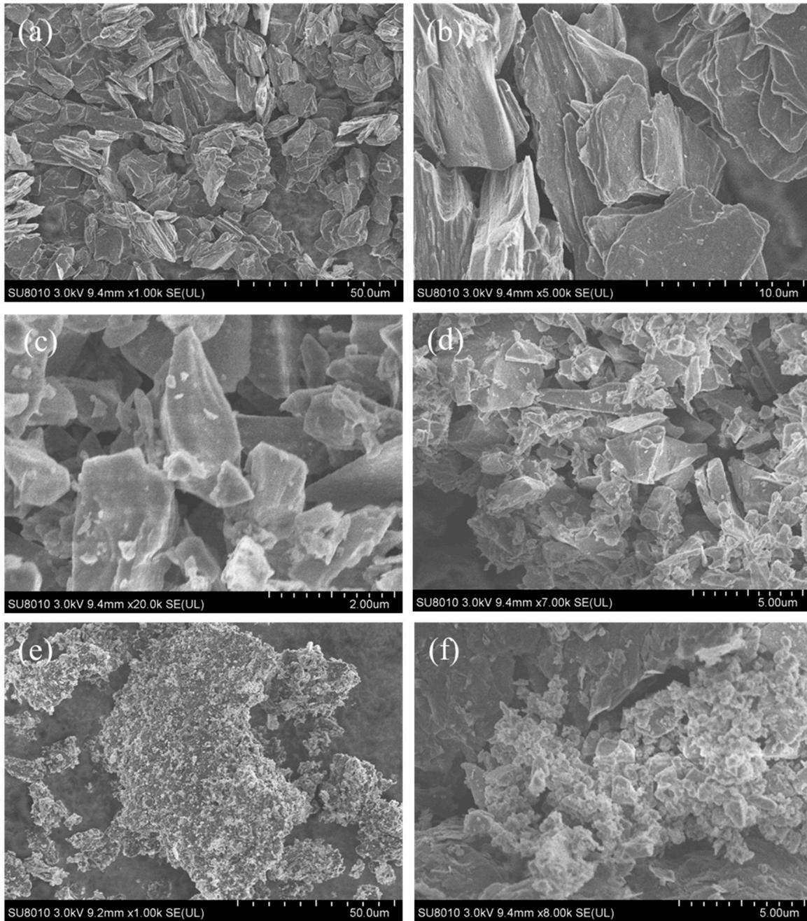
**Figure S4.** Top-down SEM of (a, b) the graphite (c, d) porous Si (e) Si@G-C composite, (f) Si/Sn@G composite.
