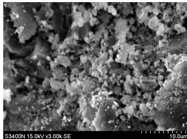
Figure 15. Microstructure 20 mm below the inner coating of the substrate (3000 $\times$ ).
