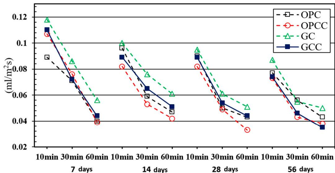
Figure 7. Comparison of the absorption rate of concrete.
