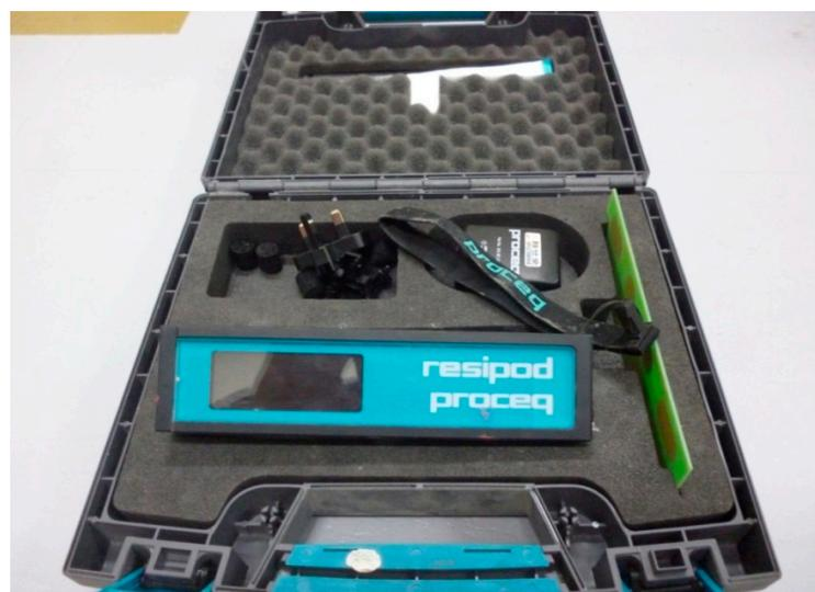
Figure 8. Four-pole resistance measuring instrument.
