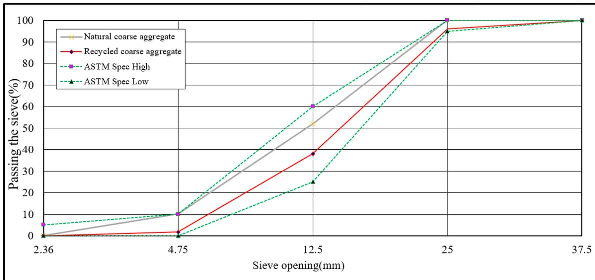
Figure 4. Particle size distribution curve of natural and recycled coarse aggregate.
