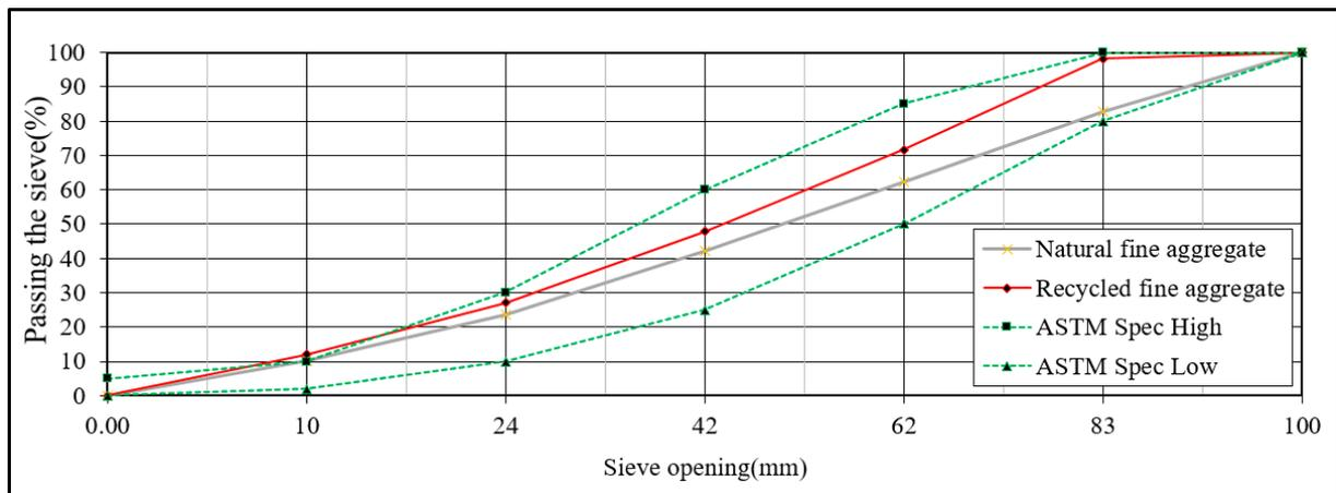
Figure 3. Particle size distribution curve of natural and recycled fine aggregate.
