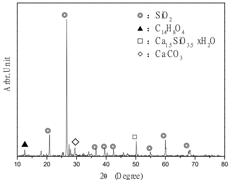
Figure 17. Chemical composition of ICM 5 mm below the coating layer, as determined through XRD.
