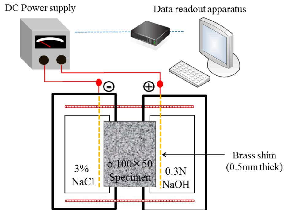
Figure 10. Schematic diagram of accelerated chloride migration test.
