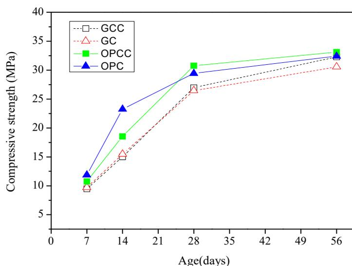
Figure 5. Compressive strength development curves.
