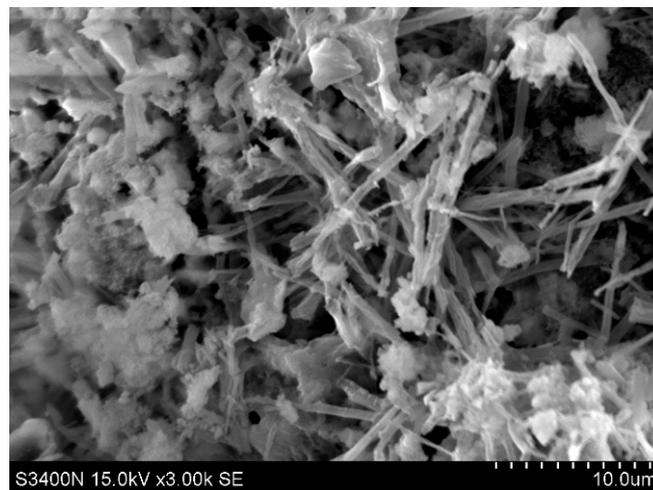
Figure 14. Microstructure 5 mm below the inner coating of the substrate (3000 $\times$ ).
