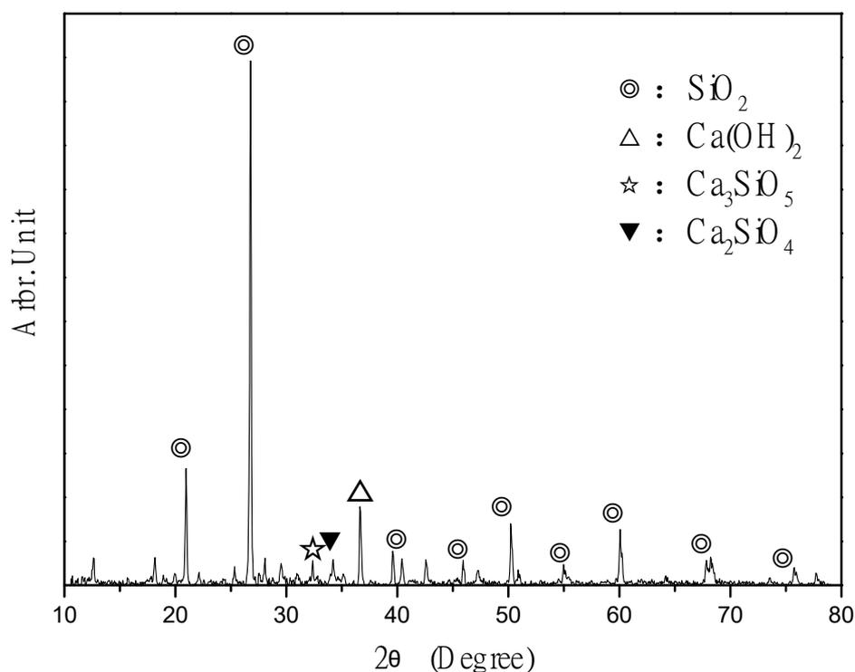
**Figure 18.** Chemical composition of pure cement substrate 20 mm below the coating, as determined through XRD.
