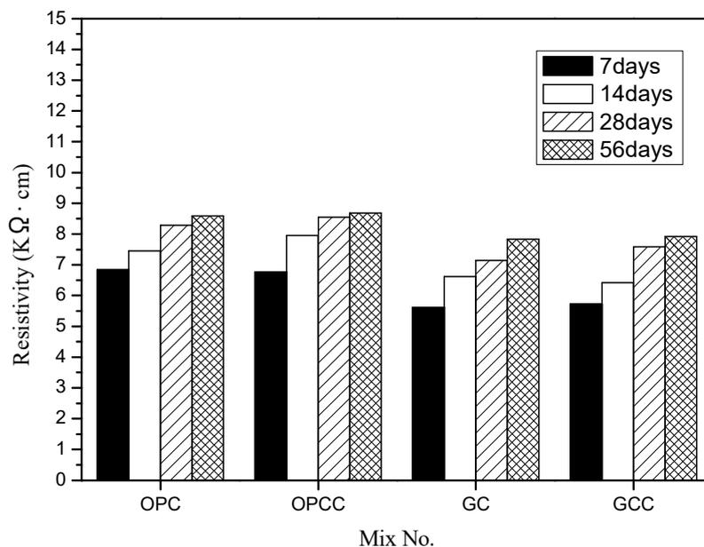
**Figure 9.** Comparison of concrete resistivity.
