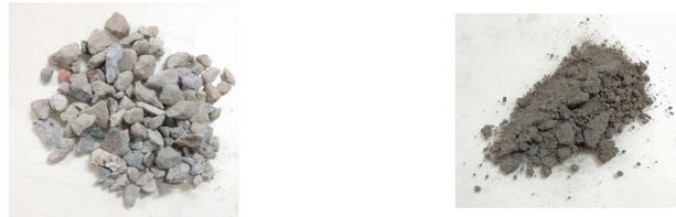
(a) Recycled coarse aggregate. (b) Recycled fine aggregate.
