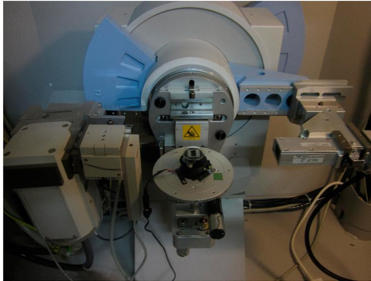
Figure 16. X-ray diffraction analyzer.
