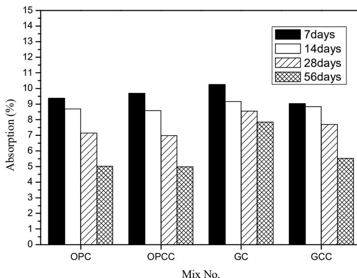
Figure 6. Comparison of absorption of concrete.
