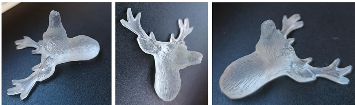
Figure S1. Photofrontally cured specimen with complex surface pattern and 3.0 cm depth, fabricated from 35 g of FPP resin R-2900_50.
