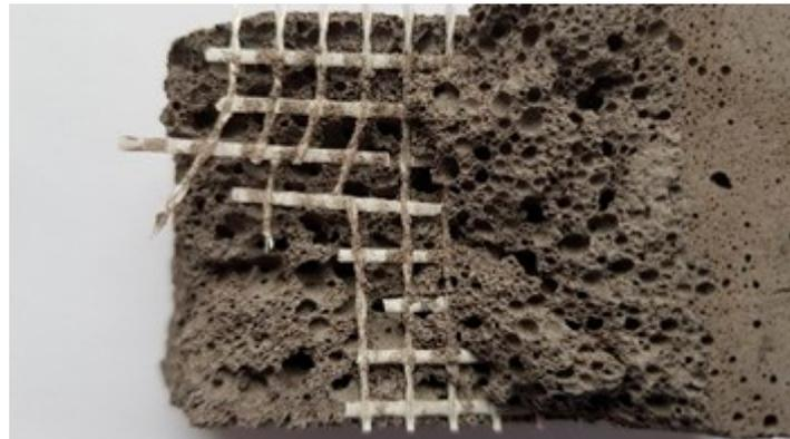
**Figure 9.** Brittle rupture of fiberglass in which the visible breakthrough does not contain free fibers.
