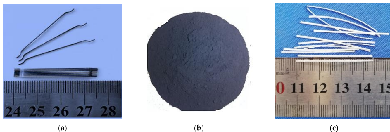
Figure 1. Dimension and shape of (a) steel fibers (b) nanocarbon black (c) polypropylene fibers.
