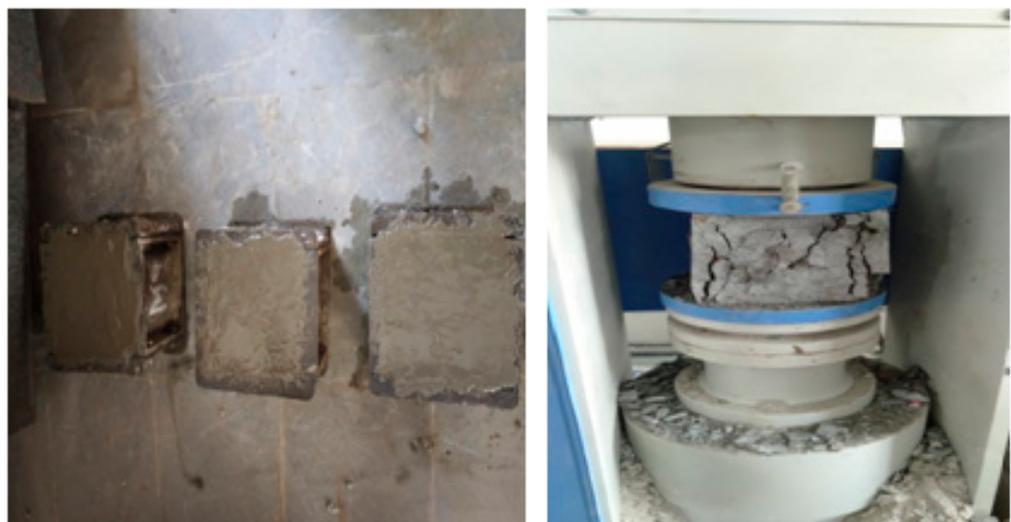
**Figure 2.** Casting and testing of CS concrete specimen.
