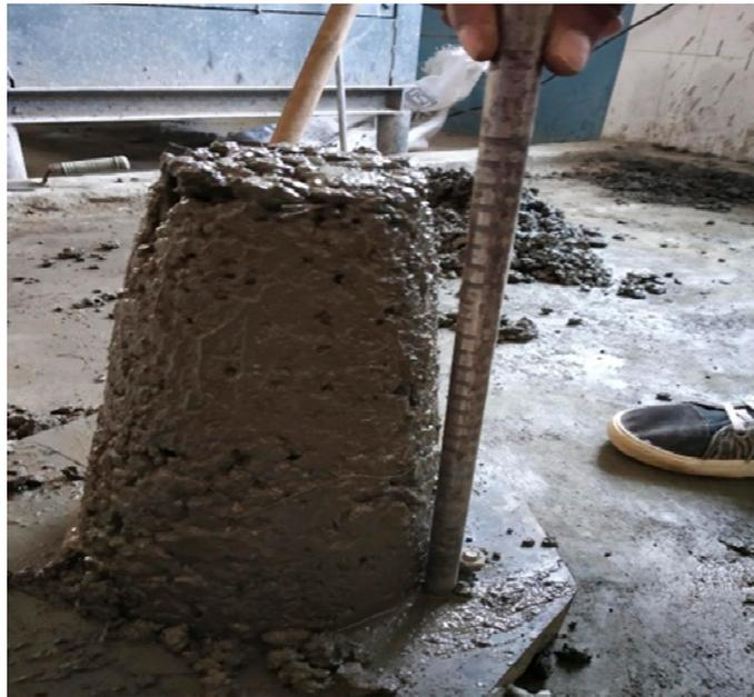
**Figure 1.** Slump of CS concrete.
