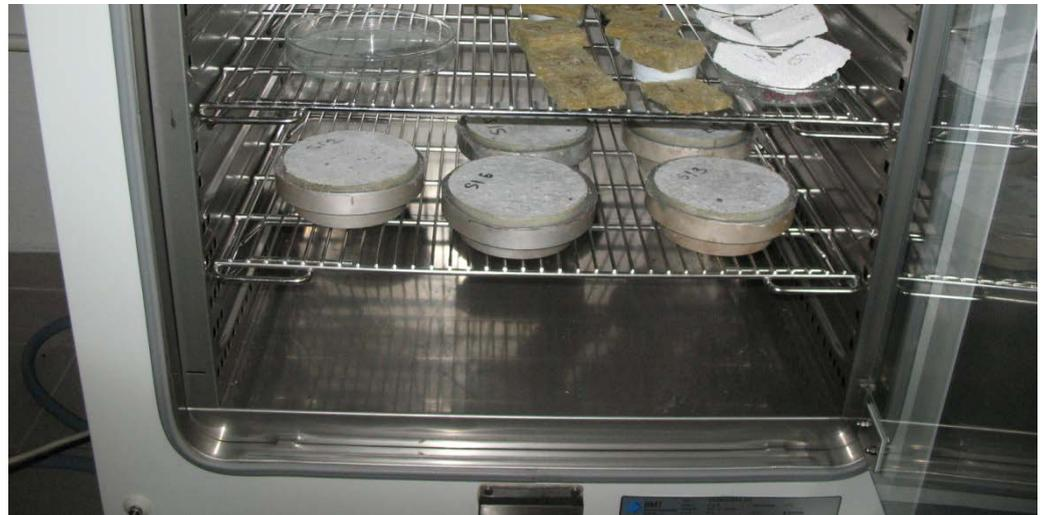
**Figure 4.** Cup method—placement of cups with samples in a climatic chamber with controlled environment.
