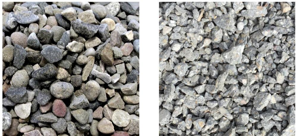
**Figure 10.** The visual comparison of particles of the natural (left) and recycled (right) coarse aggregates.
