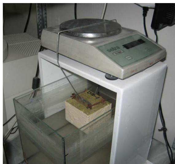
**Figure 5.** Experimental setup for the automatic measurements of water sorptivity.
