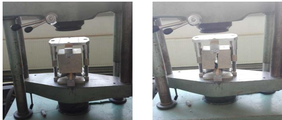
**Figure 9.** The splitting tensile strength test: a sample before (left) and after (right) the testing procedure.
