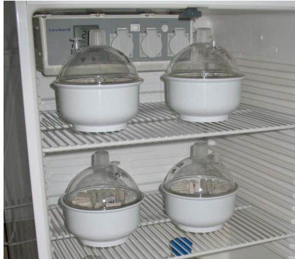
**Figure 6.** Desiccator method for measurement of the equilibrium moisture content at given relative humidity of environment.
