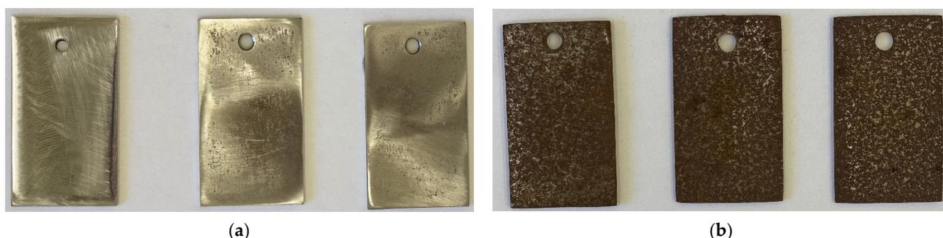
**Figure 4.** Steel samples after weathering tests for 9 months: chamber treatment with CIN vapors (a); without chamber treatment (b).
