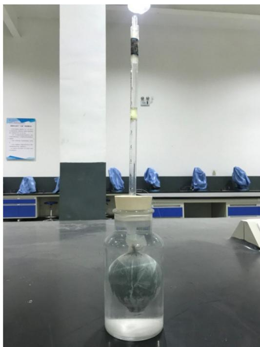
**Figure 3.** Illustration of testing set-up for the measurements of autogenous shrinkage of alkali-activated slag.
