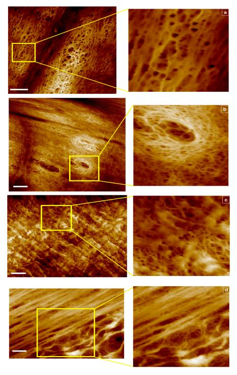
**Figure 1.** AFM images of RC membranes from top to bottom: (a) 1000 kDa in tapping mode scan area 6  $\mu m^2$ , 2  $\mu m^2$  section magnified, (b) 1000 kDa in fluid mode, scan area 8  $\mu m^2$ , 2  $\mu m^2$  section magnified, (c) 100 kDa in fluid mode scan area 8  $\mu m^2$ , 2  $\mu m^2$  section magnified, and (d) 50 kDa in fluid mode scan area 8  $\mu m^2$ , 4  $\mu m^2$  section magnified. Scale bar represents 1  $\mu m$ .
