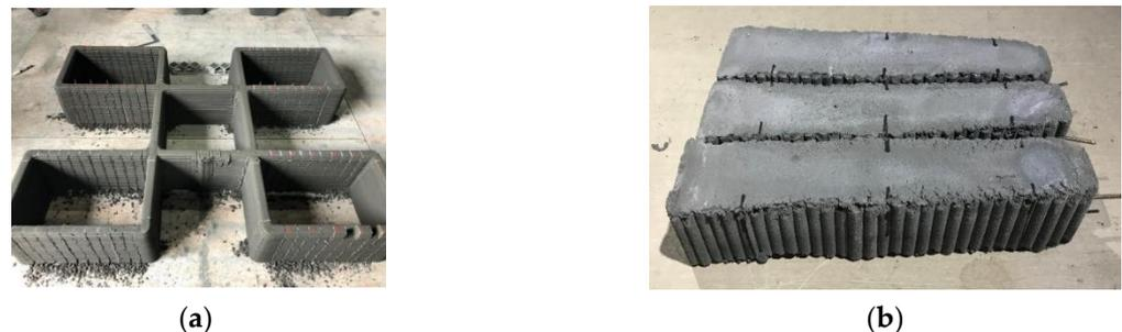
**Figure 9.** Process of extracting specimens. (a) Cutting process; (b) Cutting surface.
