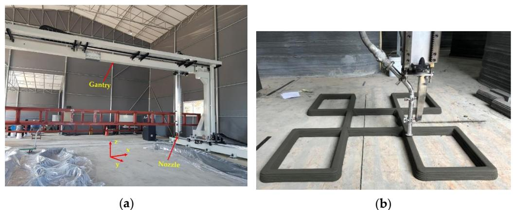
**Figure 2.** 3D-printing system. (a) Printing gantry system; (b) Printing nozzle.
