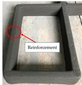
Figure 7. Penetration of reinforcements through layers.
