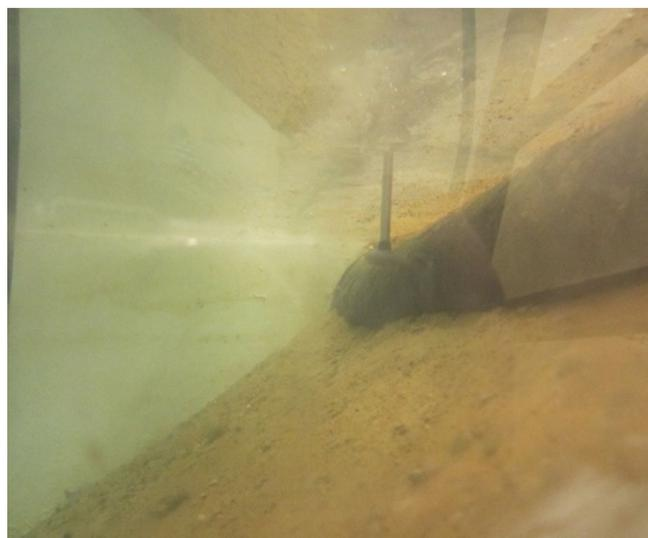
**Figure 6.** Sample flow velocity measurement at a location where water is sucked in by gravel drainage. The inlet to the drainage is protected by a geotextile against the suction of fine soil particles leading to clogging of the drainage geosynthetic.
