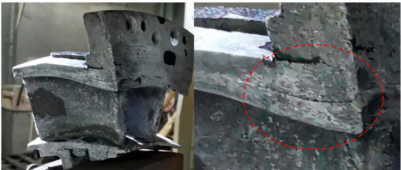
**Figure 11.** Thermal shock test of SiC/SiC twin guide vane at target temperature of  $T = 1450\text{ }^{\circ}\text{C}$  at  $N = 300$ .
