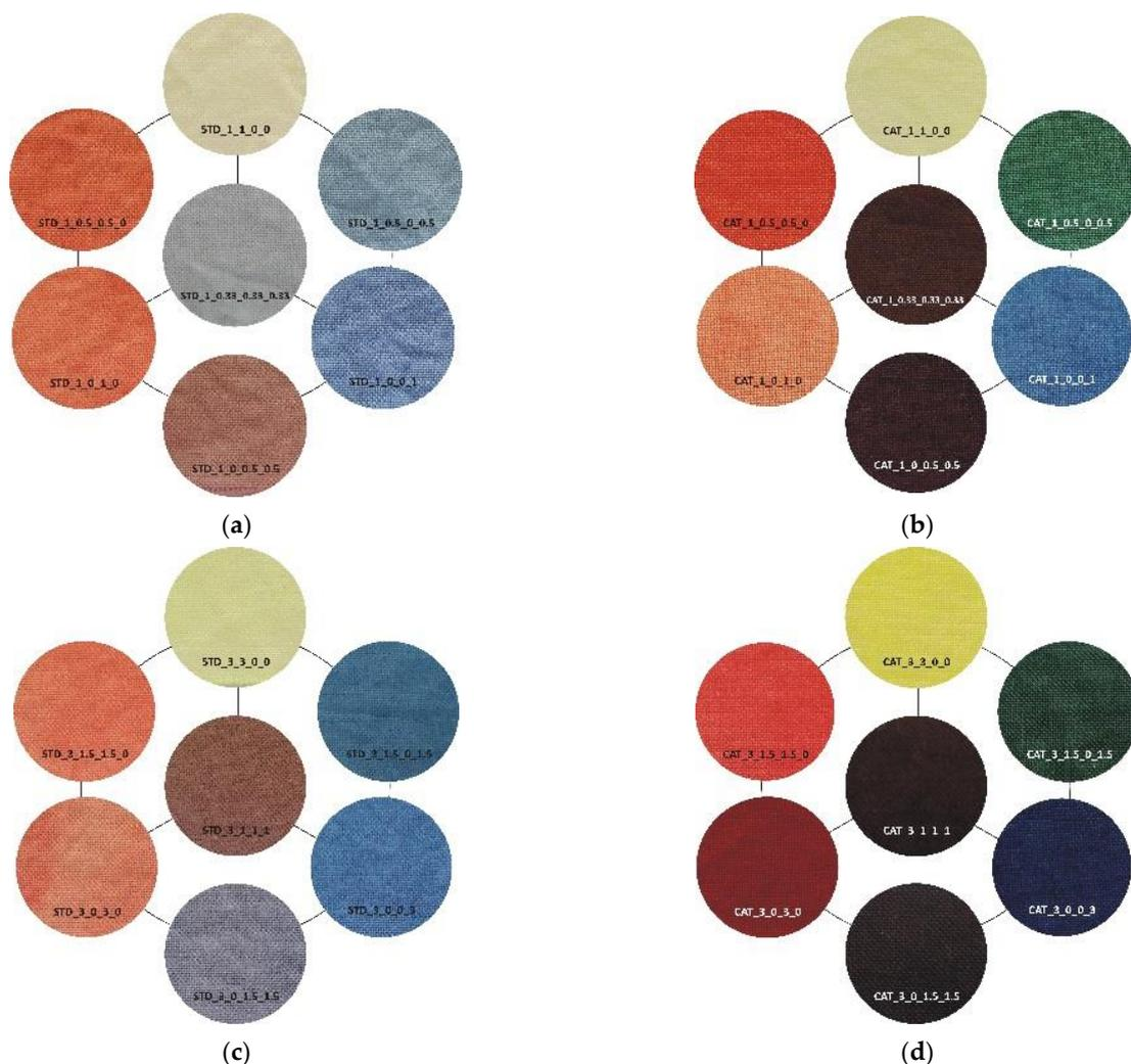
**Figure 11.** Visual representation of standard and cationized fabric dyed with vat dye: (a) Standard fabric—1% owf dye, (b) cationized fabric—1% owf dye, (c) standard fabric—3% owf dye, (d) cationized fabric—3% owf dye.
