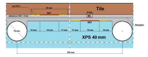
Figure 8. Vertical section II–II of the research model with C2S1 adhesive, without lamellas.
