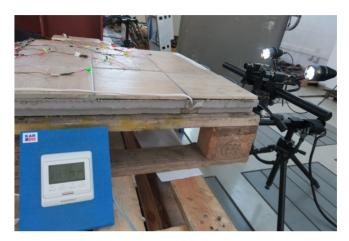
Figure 11. Aramis system test stand for measuring LFS displacements.
