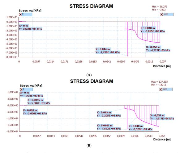
**Figure 31.** Diagram of horizontal stresses  $\sigma_x$  in the I–I section: (**A**) thermal action without ceiling deflection; (**B**) thermal action and imposed load with ceiling deflection.
