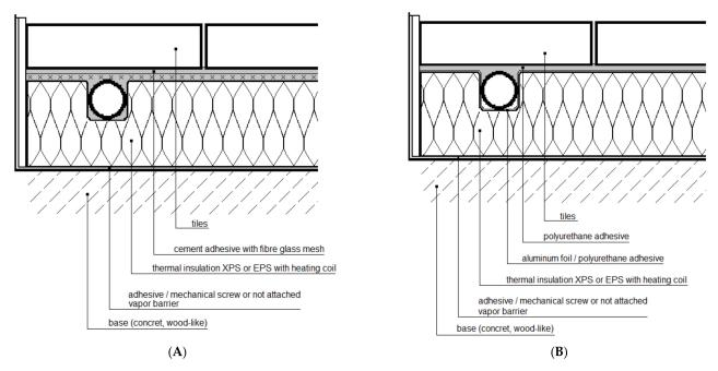
**Figure 1.** Cross-sections of a lightweight radiant heater (**A**) without a heat-dissipating layer (lamellas), and (**B**) with the heat-dissipating lamellas, namely aluminium foil.
