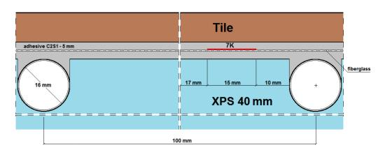
Figure 10. Vertical section IV-IV of the research model with C2S1 adhesive, without lamellas.
