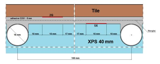
**Figure 7.** Vertical section I–I of the research model with C2S1 adhesive, without lamellas.
