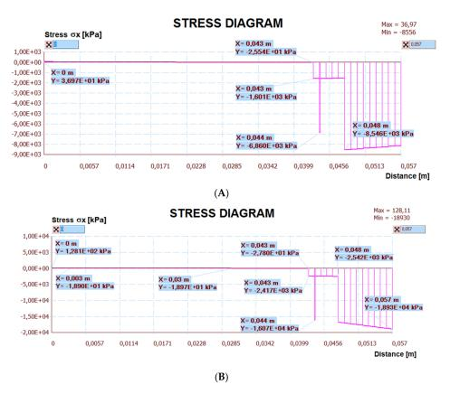
**Figure 33.** Diagram of horizontal stresses  $\sigma_x$  in the III–III section: (**A**) thermal action without ceiling deflection; (**B**) thermal action and imposed load with ceiling deflection.
