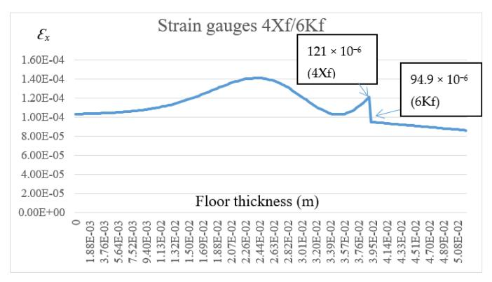
**Figure 26.** The diagram of horizontal deformations  $\varepsilon_x$  in the II–II section.
