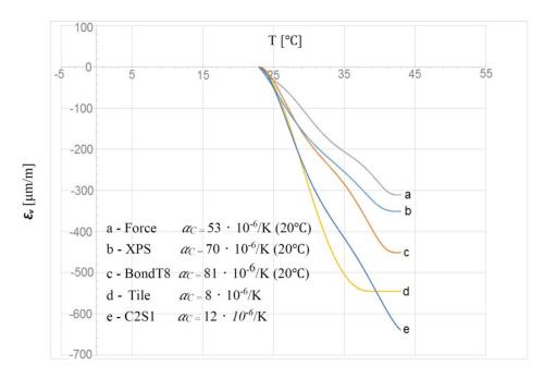
**Figure 13.** Temperature reactions of strain gauge deformation  $\varepsilon_v$  mounted on different measuring materials.
