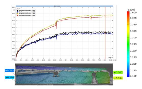
Figure 14. The number of displacements between the centre and the edge of the floor.
