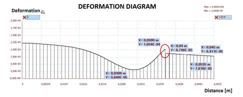
**Figure 23.** The diagram of horizontal deformations  $\varepsilon_x$  in the II–II section.
