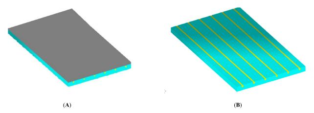
Figure 18. The 3D visualization of the model: (A) sample with an adhesive, (B) location of heating pipes.
