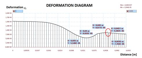
**Figure 22.** The diagram of horizontal deformations  $\varepsilon_x$  in the I–I section.
