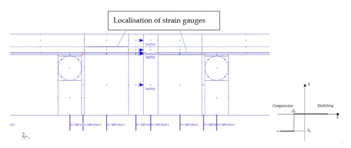
**Figure 16.** Measurement zone and substrate modelled by "contact zone". k,  $k_0$ —spring stiffness;  $\delta$ ,  $\delta_0$ —displacement.
