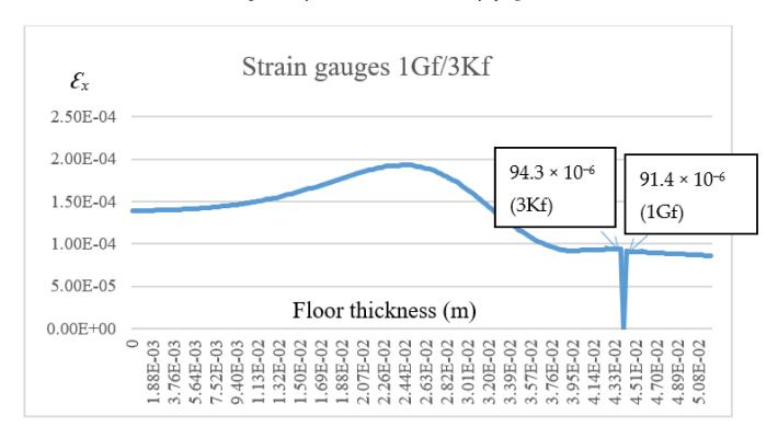
**Figure 25.** The diagram of horizontal deformations  $\varepsilon_x$  in the I–I section.
