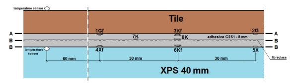
Figure 6. A and B vertical section of the research model with C2S1 adhesive, without lamellas.
