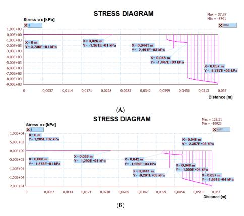
**Figure 32.** Diagram of horizontal stresses  $\sigma_x$  in the II–II section: (**A**) thermal action without ceiling deflection; (**B**) thermal action and imposed load with ceiling deflection.
