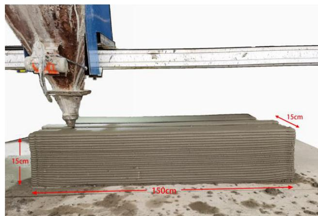
Figure 2. 3D printed cuboid.
