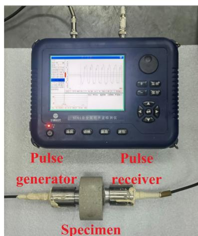
Figure 4. The UPV testing of specimens.
