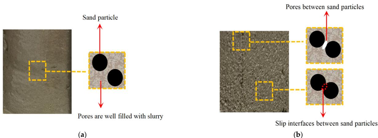
**Figure 15.** Schema of sand distribution in the internal structure. (a) With the appropriate amount of sand (b) With excess addition of sand.
